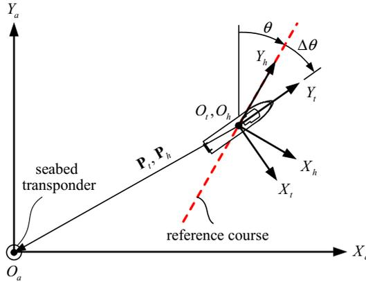
Figure 1. Vessel’s heading deviates from the course direction while conducting a USBL line survey.
