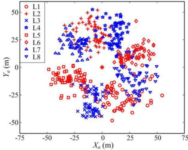
Figure 6. Seabed transponder positioning obtained directly from the raw USBL observations without misalignment correction. The asterisk is the location of the seabed transponder.
