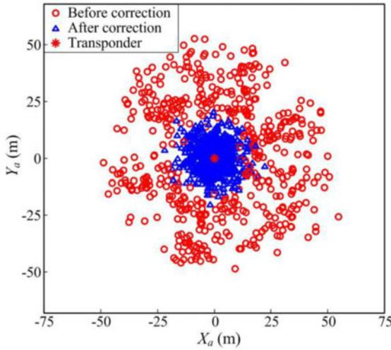
Figure 11. Position of the seabed transponder as measured with and without the correction for alignment errors, in which the estimates of roll alignment error is based on Equation (12).
