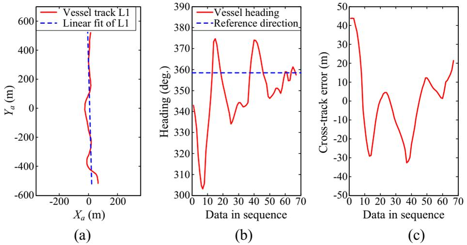
Figure 7. (a) Plot of the vessel track L1 and its linear fit in the  $O_a X_a Y_a Z_a$  coordinate system. (b) Heading of the vessel and the direction of the reference course derived from the linear fit of track L1. (c) Cross-track error of track L1.
