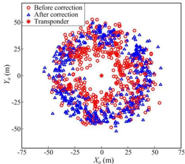
Figure 12. Position of the seabed transponder as measured with and without the correction for alignment errors, in which the estimates of roll alignment error is based on Equation (13).
