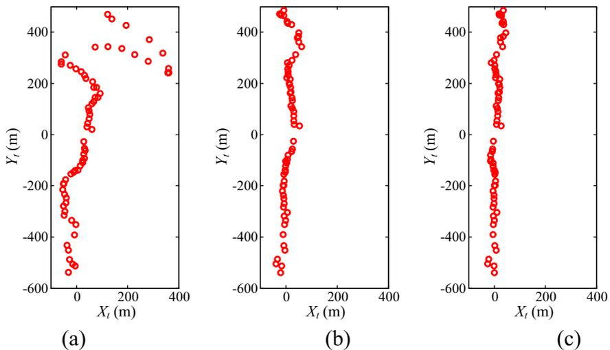
Figure 8. Corrections for heading deviation and cross-track deviation of the transponder positions observed along track L1. (a) Observed transponder positions. (b) Transponder positions after correction for heading deviation. (c) Transponder positions after corrections for heading deviation and cross-track error.
