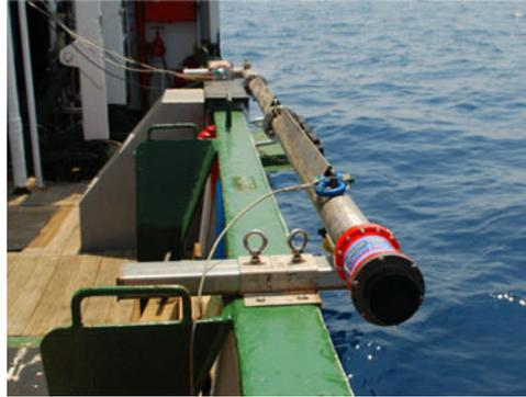
Figure 3. The USBL transceiver was installed on an over-the-side deployment pole.
