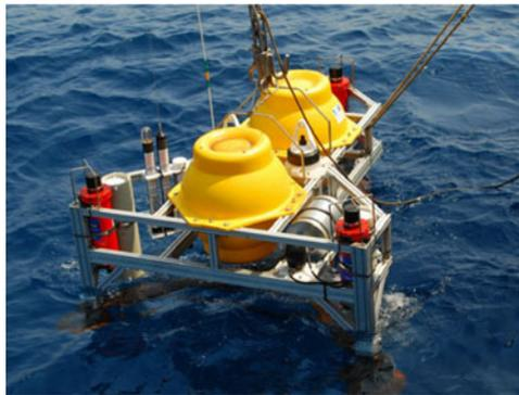
Figure 4. The Seafloor Acoustic Transponder System (SATS) was employed to carry and anchor reference USBL transponders to the seafloor.
