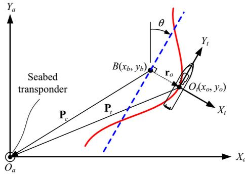
Figure 2. The vessel track and its linear fit are represented as a solid curve and a dashed line, respectively. The distance from point  $O_t$  to the reference course (dashed line) is the cross-track error.
