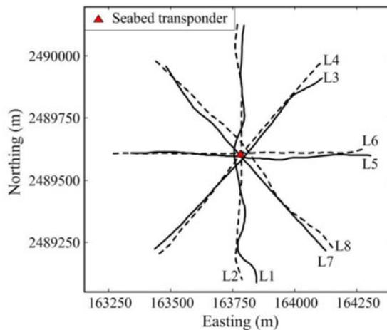
Figure 5. Vessel tracks L1-8 of the USBL line survey. The survey was centered on the reference seabed transponder that was at a depth of about 300 m.
