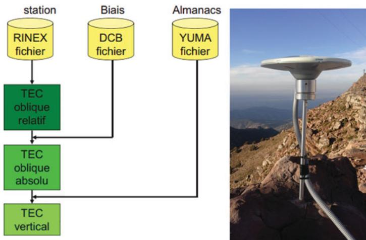
**Figure 1.** Left: Flowchart of TEC processing by Fleury model. Right: GPS at OUKAIMEDEN
