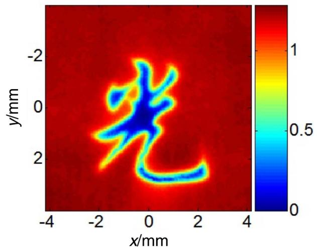
Figure 3. The measured phase distribution with the shape 光.
