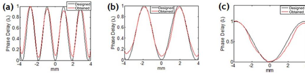
**Figure 7.** One-dimensional comparisons of designed phase distribution and measured phase distribution when the parameter  $T$  is (a) 1.86 mm, (b) 3.72 mm, and (c) 5.58 mm, respectively.
