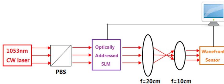
Figure 2. The optical setup for testing the optically addressed spatial light modulator (SLM). CW, continuous-wave; PBS, polarizing beam splitter.
