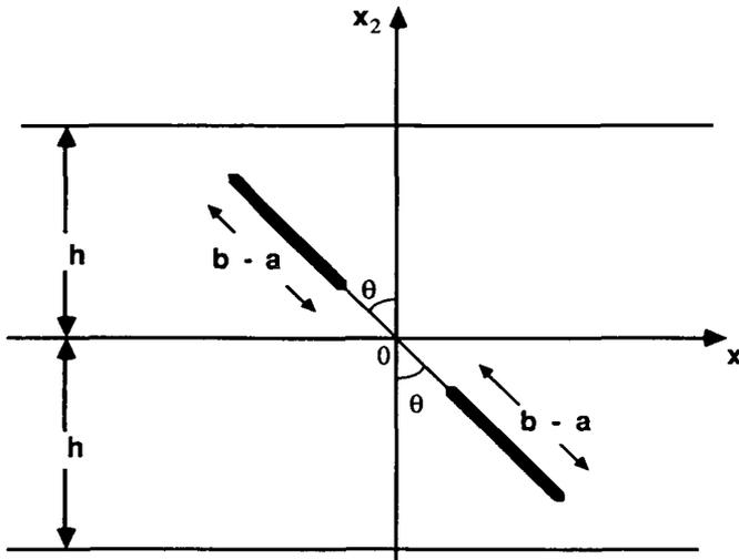
FIGURE 1. A pair of arbitrarily-oriented coplanar cracks in an anisotropic slab.
