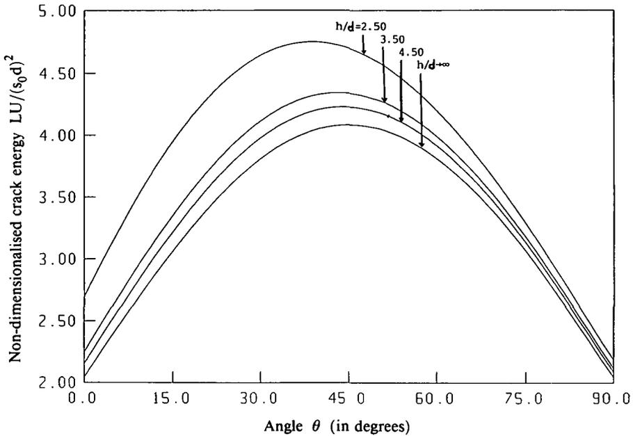
FIGURE 2. Variations of  $LU/(s_0d)^2$  with  $\theta$  for  $a/d = 0.25$ ,  $R = 1.334$  (titanium)  $h/d = 2.50, 3.50$  and  $4.50$  as well as  $h/d$  tending to infinity.
