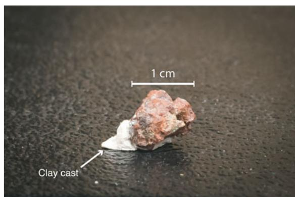
**Fig. 5.** The morphology of a typical cavity that formed along the lee side of an abrading clast, cast in clay. In the experiments presented herein, similar cavities formed sporadically but did not significantly impact basal drag.
