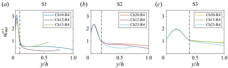
**Figure 11.** Dispersive stress  $u''_{rms}$  near S1, S2 and S3. The plots cutoff at  $y/h = 1$  or  $\langle U \rangle = \max[\langle U \rangle]$ . Here, normalization is by the friction velocity  $u_\tau$ .
