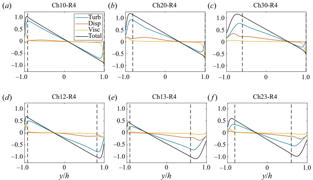
**Figure 6.** The momentum budget. The  $x$  axis is from  $y_b$  to  $y_t$  rather than from  $y_{b-}$  to  $y_{t-}$ . The dashed lines indicate the peak locations of the roughness. Turb, Disp, Visc and Total stand for turbulent flux, dispersive flux, viscous flux and total flux, respectively. Here, normalization is by the bulk friction velocity  $u_{\tau,b} = \sqrt{-1/\rho d\langle \bar{p} \rangle/dx}h$ .
