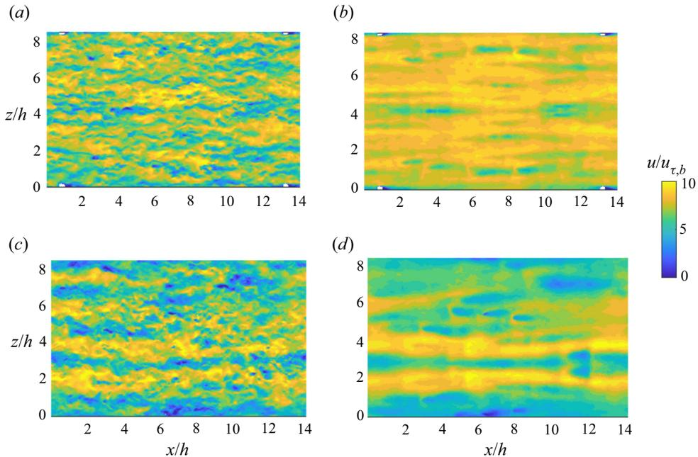
**Figure 7.** Contours of the instantaneous streamwise velocity in Ch23-R4 (a) at  $y = y_b + k_b/2$  and (c) at  $y = y_t - k_t/2$ . Contours of the time-averaged streamwise velocity in Ch23-R4 at (b) at  $y = y_b + k_b/2$  and (d) at  $y = y_t - k_t/2$ .
