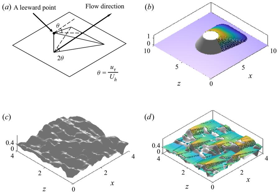
**Figure 17.** (a) A sketch of the sheltering behind a leeward point. (b) A sketch of the sheltering behind a frustum. (c) A cut from S3. (d) Flow sheltering on the roughness in (c). The flow is from the  $-x$  to the  $+x$  direction.
