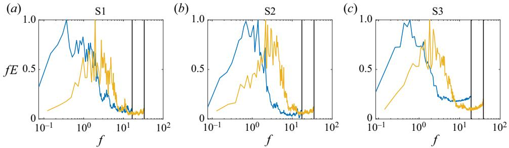
**Figure 5.** Premultiplied roughness spectra. The spectra are normalized by their maxima. The blue lines are the  $x$  direction spectra. The yellow lines are the  $z$  direction spectra. The vertical lines denote the grid cutoff in the  $Re_\tau = 395$  DNSs.
