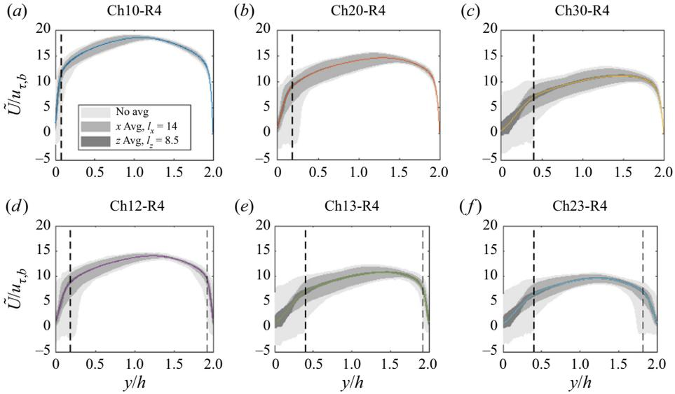
**Figure 12.** Mean velocity. The shades show the variation of the mean velocity when the data are not subjected to any spatial filtration, when the data are subjected to streamwise filtration of  $l_x = 14h$  and when the data are subjected to spanwise filtration of  $l_z = 8.5h$ .
