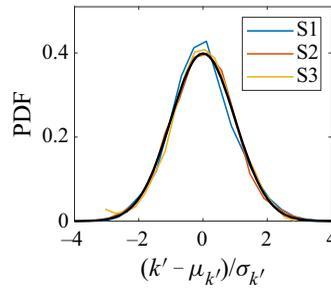
**Figure 3.** The probability density function (PDF) of the roughness height distribution. Here,  $\mu_{k'}$  is the mean roughness height, and  $\sigma_{k'}$  is the standard deviation of the roughness height. The black solid line is the standard Gaussian distribution.
