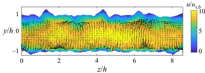
**Figure 8.** Contours of the time-averaged streamwise velocity at a constant  $x$  location. The arrows show the in-plane motion. For visualization purposes, we show arrows between  $y = k_b/2$  and  $y = 2 - k_t/2$  only.
