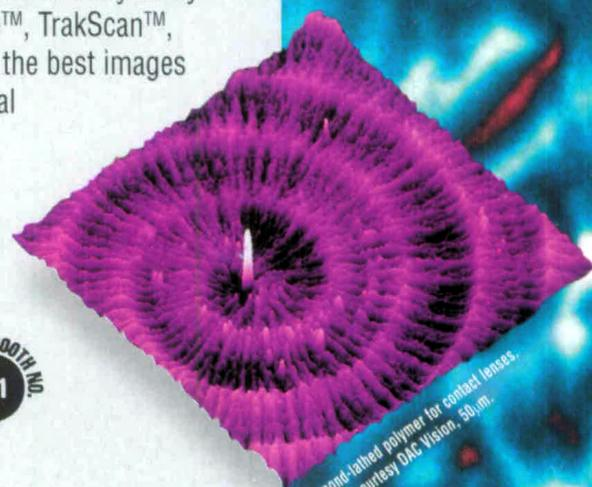
Diamond-tipped polymer for contact lenses. Sample courtesy DAC Vision, 50 μm.
