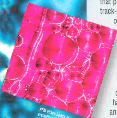
AFM phase image of liquid crystalline dendrimer showing birefringent "fan"-like domains\*
