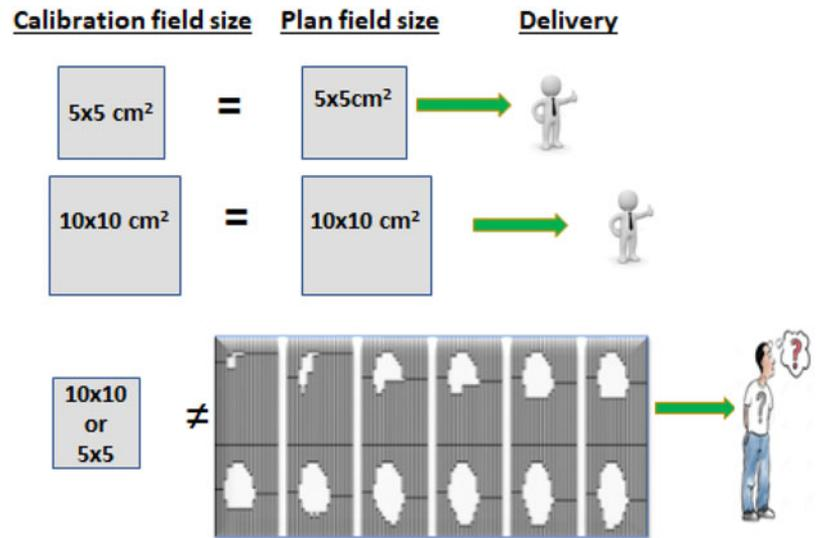
**Figure 1.** Simple calibration square field not true representation of the true complex segments of the VMT/IMRT plans
