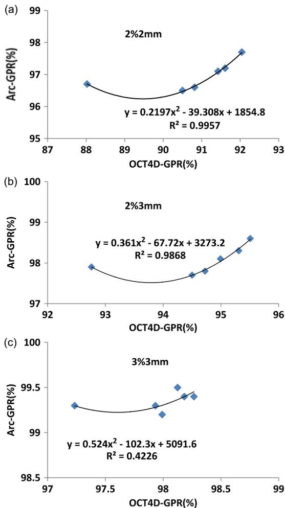
**Figure 4.** (a), (b), (c): Correlation of GPR between 4DOCT and Arc Check for (a = 2% 2mm, b = 2%3mm and c = 3%3mm)
