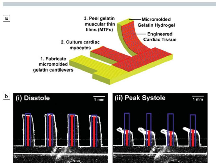
(a) Fabrication of gelatin muscular thin films; (b) Optical micrographs of voltage-paced muscular thin film cantilevers in which the muscle tissue is either in a relaxed ("diastole") or contracted ("systole") state. Reproduced with permission from *Biomaterials* **35** (2014) DOI: 10.1016/j.biomaterials.2014.03.052; p. 5462. © 2014 Elsevier Ltd.
