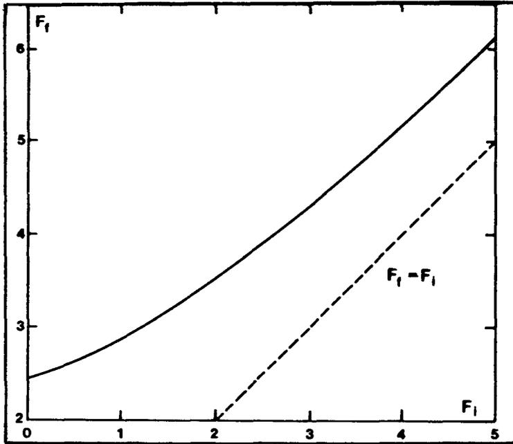
figure 6 : the free vibration amplitude after transition ( $F_f$ ) versus its value ( $F_i$ ) before transition for a passage through resonance with decreasing  $\delta$  (for internal circulation orbits).
