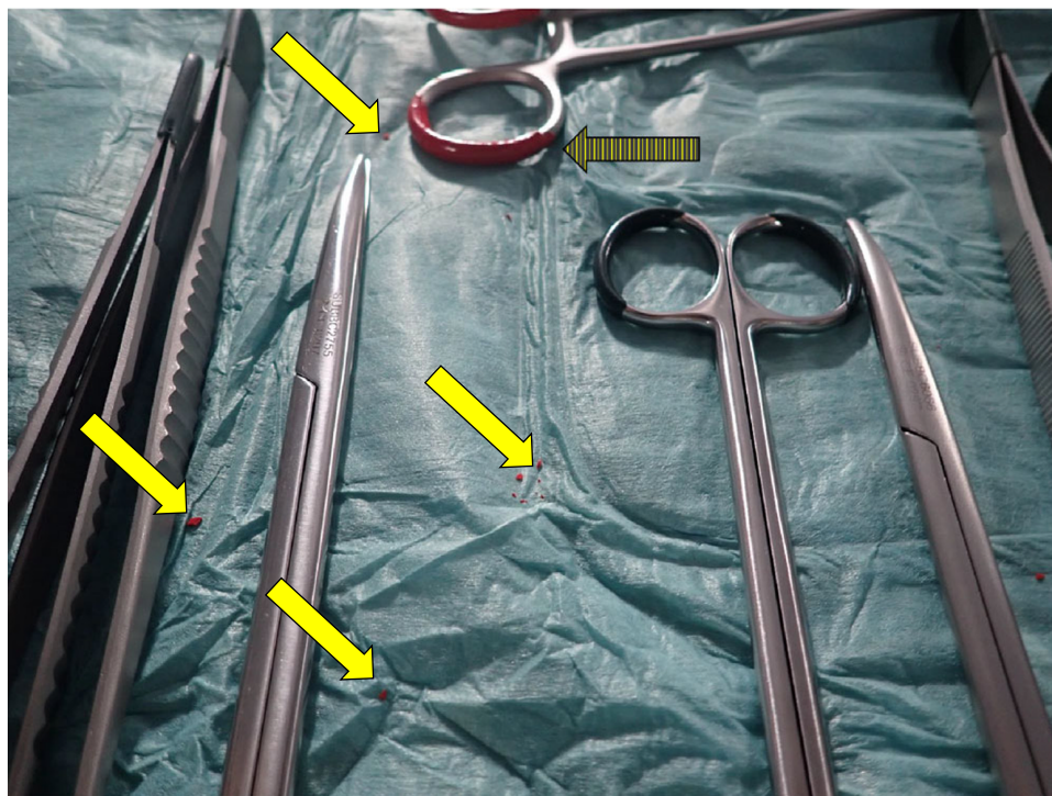
Figure 6. New, unused SI in its original packaging. The red color, which is applied as a label and safety marking, is crumbling away (black-yellow striped arrow). The crumbs are distributed over the other SI (yellow plain arrows).
