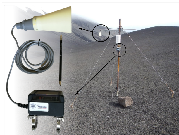
Figure 2. Photograph of one of the monitoring stations showing the installation setting of a MB7574-SCXL-Maxsonar MaxBotix ultrasonic sensor with the protective cone attached, at the end of a horizontal mast to keep a > 75 cm distance from the main mast where the Geoprecision-Box datalogger was installed to avoid interference and erroneous distance measurements to the ground surface.
