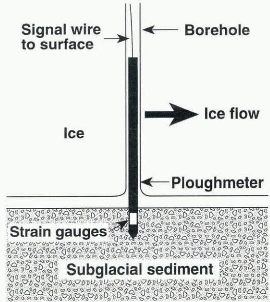
Fig. 2. Schematic diagram showing a ploughmeter installed at the glacier bed. The ploughmeter is hammered into basal sediments such that the upper part becomes trapped within glacier ice. Strain gauges bonded to the immersed section respond to elastic bending of the ploughmeter as the device is dragged through basal sediments by the motion of the glacier.
