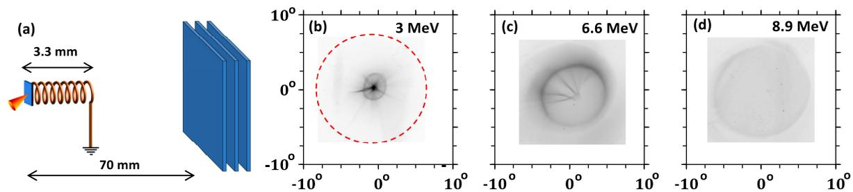
**Figure 4.** (a) shows a schematic of the setup used for the shot taken with a 3.3 mm long helical coil with RCF placed at 70 mm from the interaction foil. (b), (c) and (d) show the raw RCF images for 3.0, 6.6 and 9.6 MeV protons respectively, where the pronounced focusing of the channelled beam of 3 MeV protons can be seen in (b), in contrast to the geometrical projection of the exit winding of the coil at the RCF plane shown by the red dashed circle.
