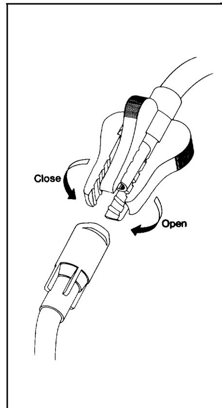
Male connector protected by overlapping ribs. Threads on the underside of the rib: engage with the standard female Luer connection.
