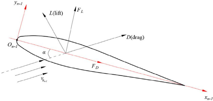
Figure 16. Schematic analysis of the stress of the caudal fin.
