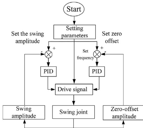
Figure 13. Joint closed-loop control flowchart.
