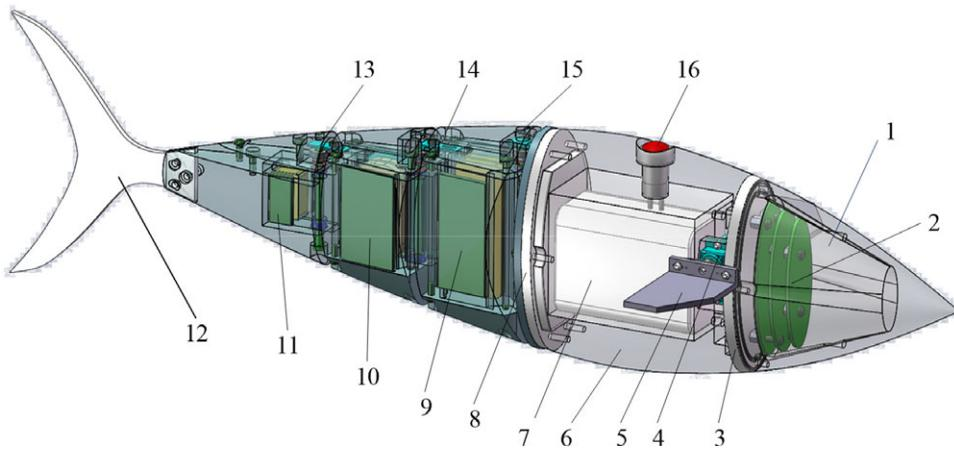
**Figure 19.** Three-dimensional structure of bionic tuna:(1) fish head, (2) control circuit board, (3) fish head waterproof board, (4) pectoral steering gear, (5) pectoral fin, (6) battery compartment, (7) battery, (8) battery waterproof plate, (9) first joint, (10) second joint, (11) third joint, (12) caudal fin, (13) third angle sensor, (14) second angle sensor, (15) first angle sensor, and (16) waterproof switch.
