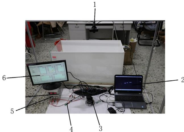
**Figure 21.** Bionic tuna experimental equipment: (1) IR camera, (2) camera data acquisition end, (3) bionic tuna, (4) serial communication module, (5) power, and (6) LabVIEW data acquisition host.
