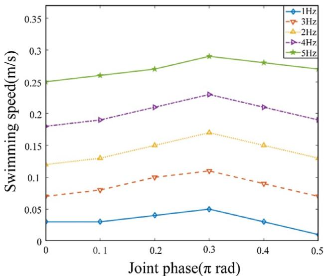
**Figure 18.** Swimming speed of bionic fish under different frequencies and phase differences.
