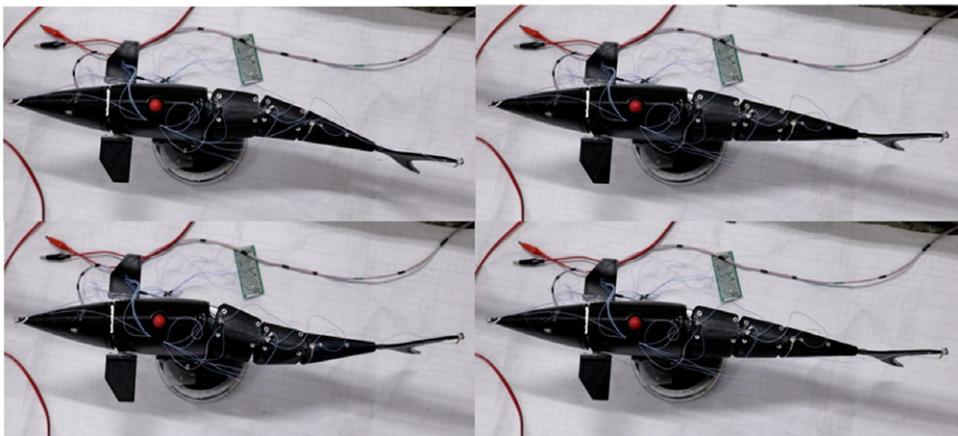
Figure 24. Illustration of head and tail fin swing attitude of bionic tuna ( $F = 4\text{Hz}$ ,  $\varphi = 0.2$ ).
