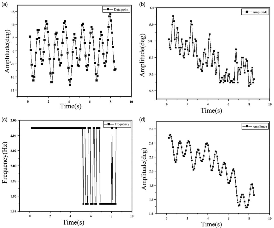
**Figure 12.** Open-loop joint test data: (a) joint swing curve, (b) swing amplitude, (c) swing frequency, and (d) zero offset.
