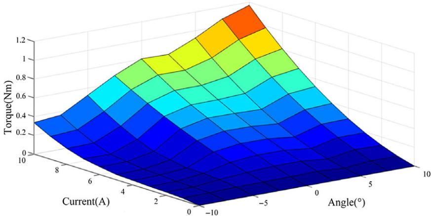
**Figure 9.** Simulation diagram of the relationship between single coil and rotation angle current and torque.
