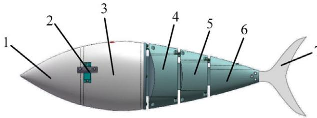
**Figure 1.** Outline of bionic fish: (1) fish head, (2) pectoral fin, (3) fish body, (4) the first drive joint, (5) the second drive joint, (6) the third drive joint, and (7) caudal fin.
