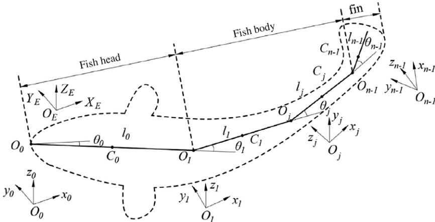
Figure 15. Coordinates of the bionic tuna system.
