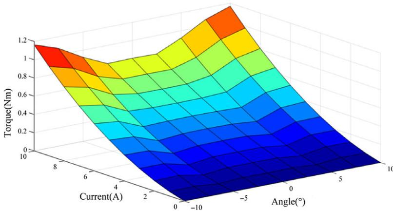
*Figure 10. Torque diagram of the dual coil using mode one.*
