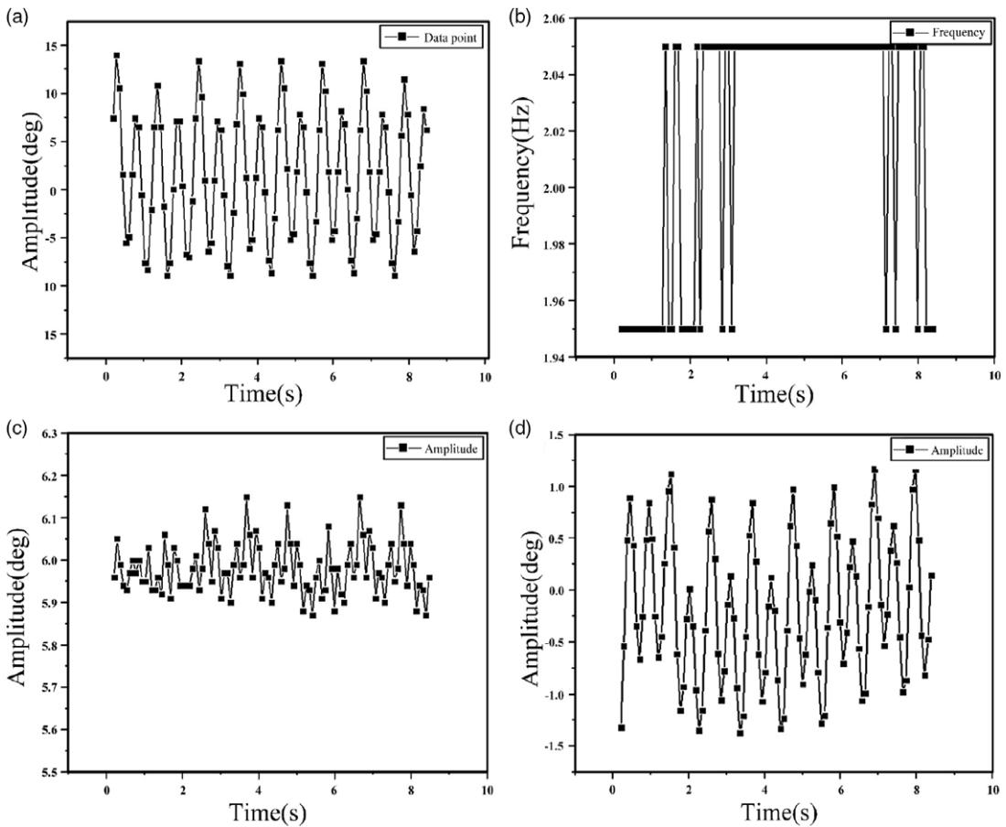
**Figure 14.** Joint closed-loop test data: (a) joint swing curve, (b) swing frequency, (c) swing amplitude, and (d) zero offset.
