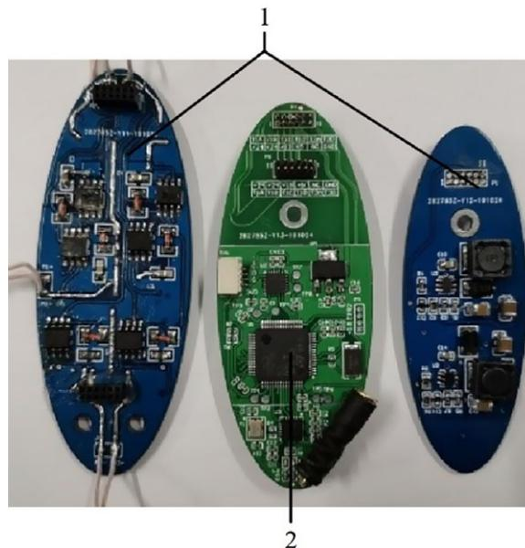
**Figure 20.** Bionic fish control hardware system: (a) joint electromagnetic-driven control circuit board and (b) main control chip and pose measurement control circuit board.
