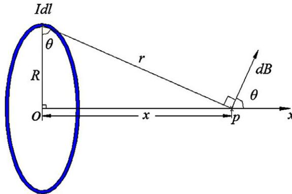
Figure 2. The electromagnetic field generated by a ring current.
