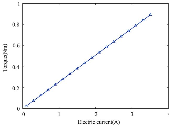
**Figure 7.** Relation curve of joint thrust and current.
