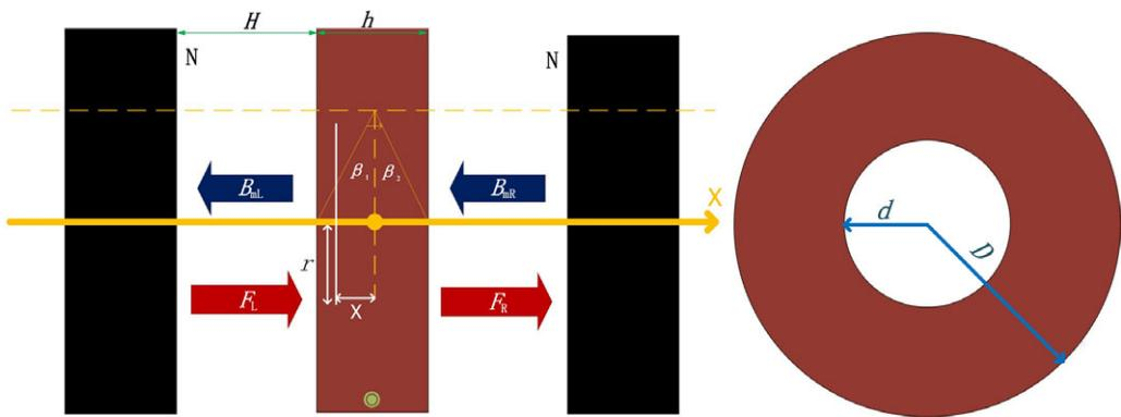
Figure 3. Schematic diagram of the electromagnetic drive.
