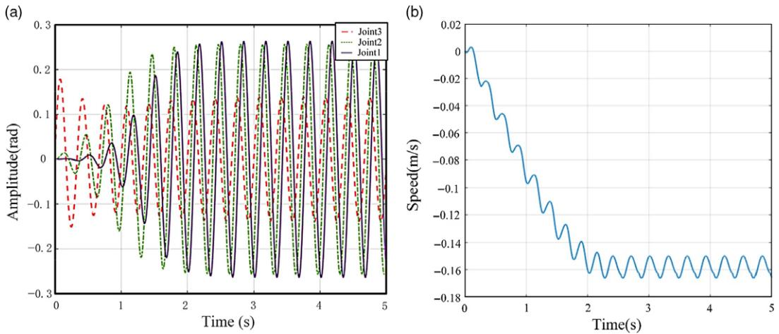
**Figure 17.** Kane kinetic simulation curve of bionic tuna: (a) CPG control curve and (b) bionic fish swimming speed.
