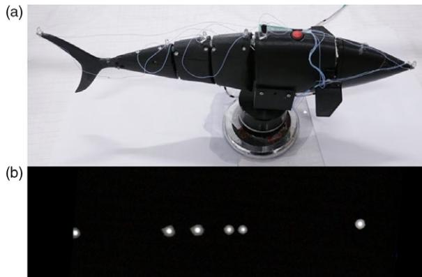
**Figure 22.** Experimental device of motion attitude measurement: (a) bionic tuna prototype and (b) infrared detection pose state.
