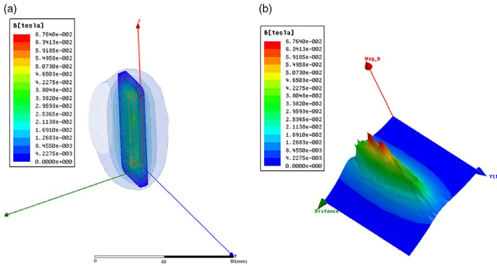
**Figure 6.** Finite element simulation results of magnetic field strength of electrified coil: (a) three-dimensional magnetic field intensity distribution and (b) distribution of magnetic field intensity of electrified coil.
