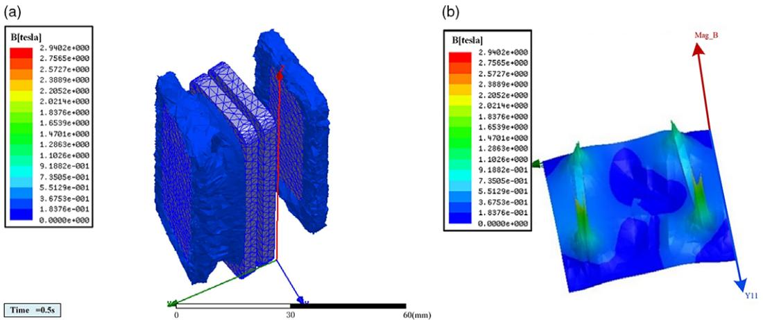
**Figure 8.** Bionic fish first joint simulation diagram: (a) simplified structure of the first joint of bionic fish and (b) bionic fish first joint electromagnetic strength.
