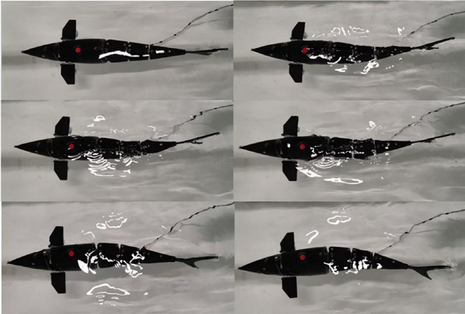
**Figure 26.** Motion sequence diagram of bionic tuna prototype in underwater linear cruise.
