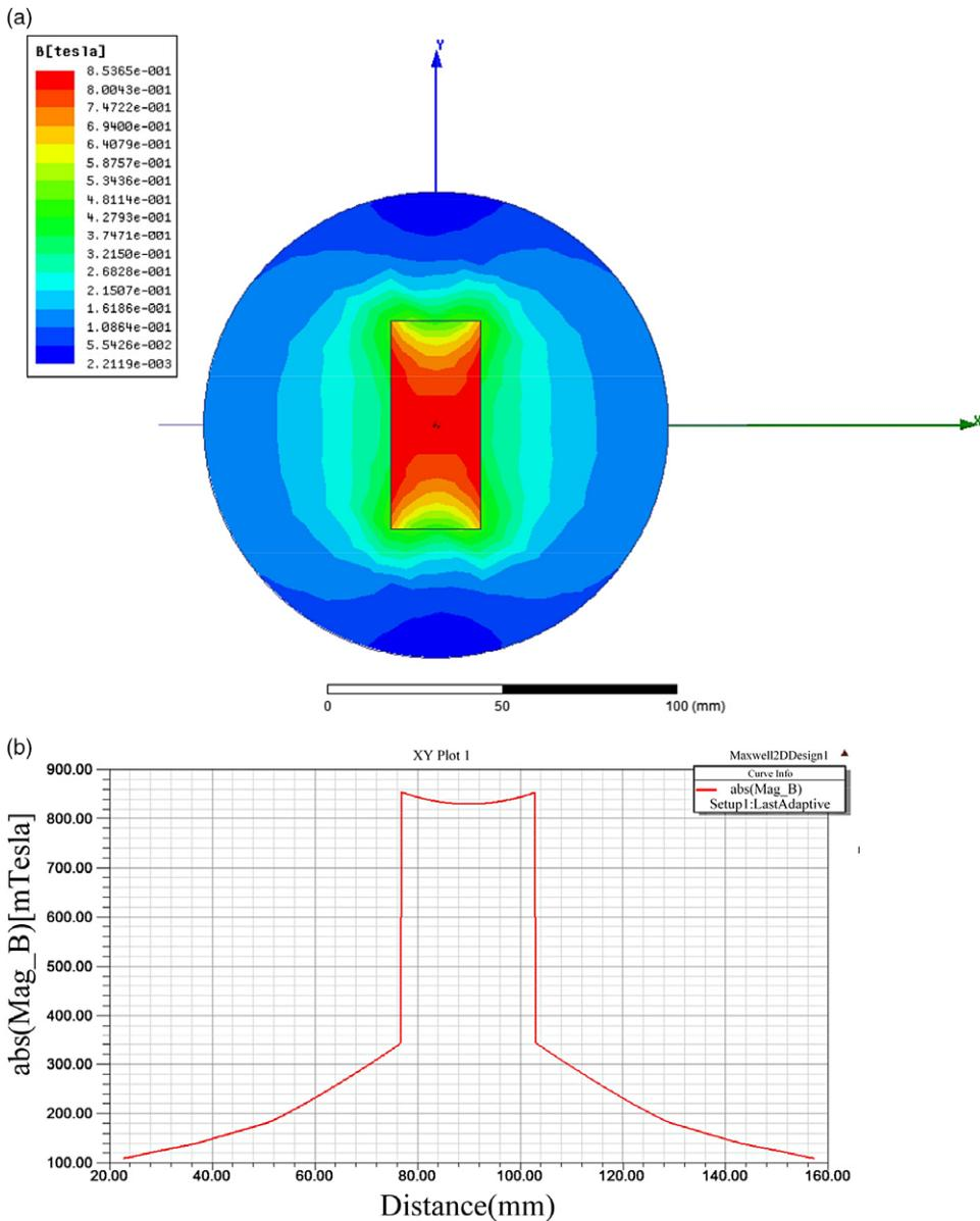
**Figure 5.** Finite element simulation results of permanent magnet magnetic field strength: (a) magnetic field distribution of magnet and (b) magnetic field intensity position curve of magnet.
