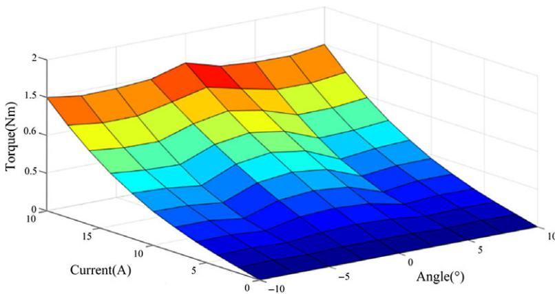
*Figure 11. Torque diagram of the second coil using mode two.*
