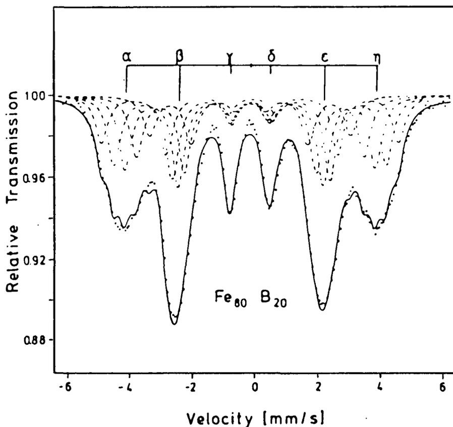
Figure 6. Mössbauer spectrum of the amorphous metal  $\text{Fe}_{80}\text{B}_{20}$ . The stick diagram ( $\alpha, \beta, \sigma, \delta, \epsilon, \eta$ ) represents the average hyperfine field. The solid line represents the sum of the subspectra.<sup>10</sup>
