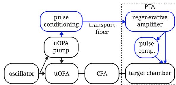
**Figure 1.** Scheme of the principle of the SEPPL (blue boxes) integrated into the PHELIX facility (black boxes). It shows the main components of the SEPPL, namely the pulse conditioning, amplification, pulse compression and transport of the pulse.
