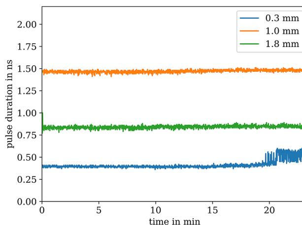
**Figure 6.** Pulse duration stability over 23 minutes for different FPC lengths. Only the shortest cavity shows a deviation after 10 minutes.
