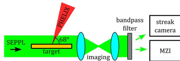
**Figure 7.** Experimental setup using the SEPPL as a probe laser for the characterization of a preplasma induced by the PHELIX laser. The probe can be sent into an MZI for measuring the density profile or used for streaked shadowgraphy of the plasma expansion.
