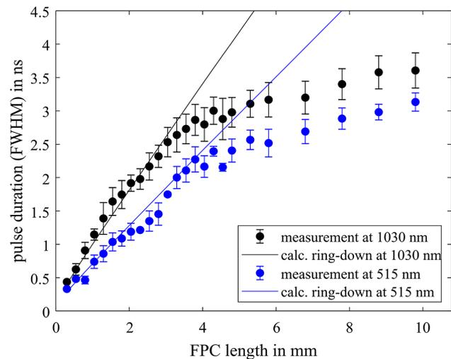
**Figure 4.** Dependency of the pulse duration at 1030 nm (black) and 515 nm (blue) on the length of the FPC used for the seed generation. The black and blue lines correspond to the calculated pulse duration at central wavelengths of 1030 and 515 nm, respectively, given by the cavity ring-down using a reflectivity of 99.7% for both mirrors.
