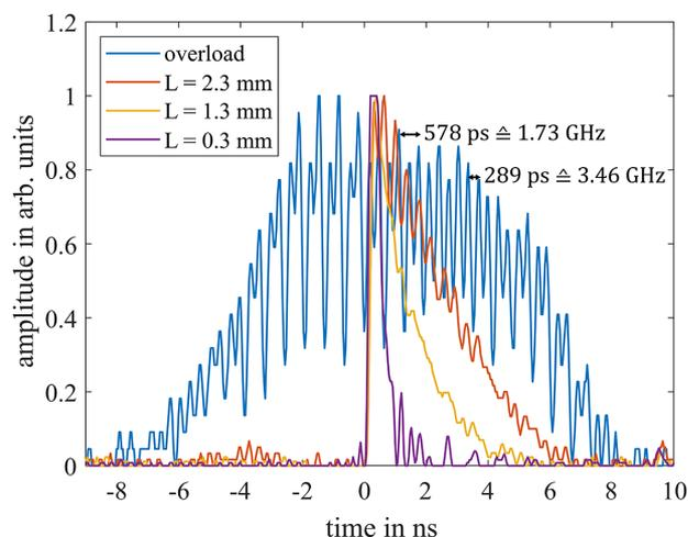
**Figure 5.** Shape of the pulse duration using FPC distances of 0.3 mm (purple), 1.3 mm (yellow) and 2.3 mm, as well as the resulting pulse using the overload (OL) mode of the amplification cavity (blue).
