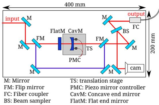
**Figure 2.** Schematic drawing of the seed-pulse conditioning. The incoming pulse can be sent into the FPC (dark blue mirrors), which can also be bypassed before sending the output pulse into the fiber coupler. In addition, a sample of the FPC transmission is monitored on a camera to control the cavity alignment.
