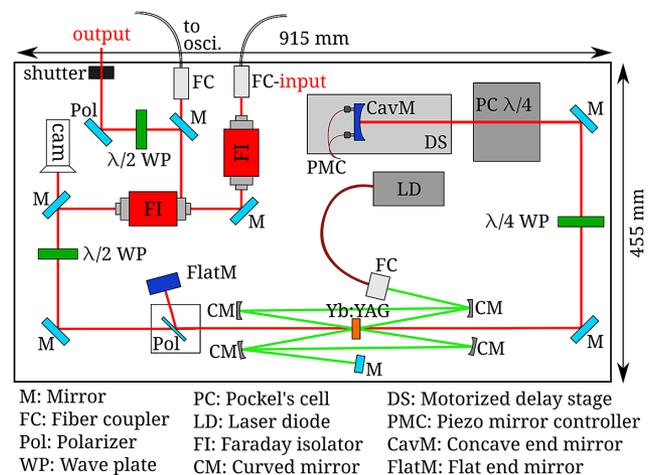
**Figure 3.** Schematic drawing of the regenerative amplifier with a total size of 915 mm × 455 mm. The input pulse enters the amplifier through a fiber coupler (red input), passes two Faraday isolators and enters the main cavity, delimited by the flat and concave mirrors (blue). The cavity is set up around a Yb:YAG crystal, which is being pumped by a 12-pass pump system, powered by a laser diode.
