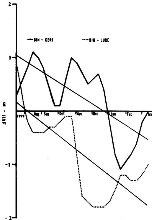
Figure 1. UT1-UTC residuals from connected-element interferometer (CERI) and lunar ranging (LURE).
