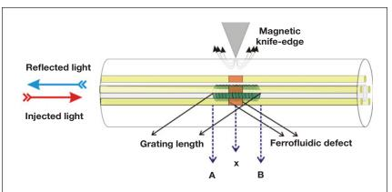
A schematic of the microfluidic optical fiber in which an infiltrated ferrofluid (orange) alters the spectrum reflected from a Bragg grating (green). Reproduced with permission from *Opt. Lett.* **36**(13)(2011), DOI:10.1364/OL.36.002548, p. 2548. © 2011 Optical Society of America.
