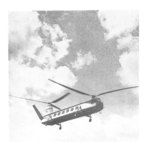
The Bristol 173 Helicopter is fitted with two Alvis Leonides Engines
