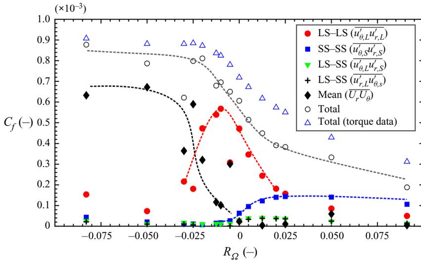
FIGURE 5. Contributions to the friction factor  $C_f$  associated with the mean flow and the instantaneous large-scale (LS) and smaller-scale (SS) velocity fluctuations in the TC gap at  $Re_S = 29000$ . Their combined total (circles) is compared against the estimated based on the torque measurements of Ravelet *et al.* (2010) (triangles). The dashed lines are indicative of the trend in the data.
