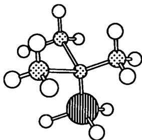
**TMAA is a new source reagent for growth of AlGaAs by MOCVD and MOMBE with dramatically reduced carbon and oxygen levels when compared to growth using trialkylaluminums. TMAA is not pyrophoric and its high vapor pressure and low decomposition temperature allow for high growth rates at a wide range of temperatures.**
