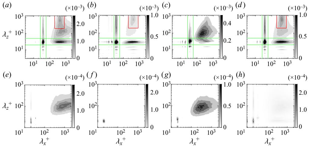
Figure 15. Premultiplied two-dimensional spectral densities: (a,e)  $k_x k_z E_{uu}$ ; (b,f)  $k_x k_z E_{vv}$ ; (c,g)  $k_x k_z E_{ww}$ ; (d,h)  $k_x k_z E_{uv}$  at  $y^+ = 0$ . Here (a–d) HP1; (e–h) LP1. The red lines demarcate  $200 \lesssim \lambda_x^+ \lesssim 800$  and  $200 \lesssim \lambda_z^+$ . The green lines enclose the signature of the pore-coherent flow which are coincident with  $\lambda_x^+ = s_x^+$  and  $\lambda_z^+ = s_z^+$ .
