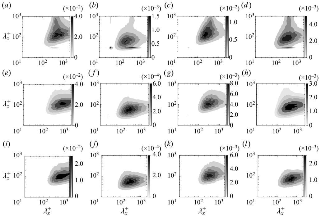
Figure 12. Pre-multiplied two-dimensional spectral energy densities: (a,e,i)  $k_x k_z E_{uu}$ ; (b,f,j)  $k_x k_z E_{vv}$ ; (c,g,k)  $k_x k_z E_{ww}$ ; (d,h,l)  $k_x k_z E_{uv}$  at  $y^+ \approx 5$ . Here (a–d) HP1; (e–h) MP; (i–l) LP1.
