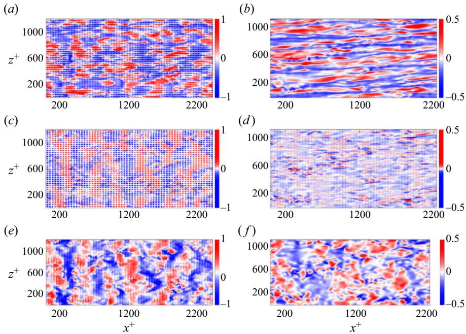
Figure 14. Instantaneous fluctuations of (a,b) streamwise velocity, (c,d) wall-normal velocity and (e,f) pressure at  $y^+ = 0$ . Here (a,c,e) HP1; (b,d,f) LP1. Flow direction is from left to right. The white regions represent the solid rods of the substrate.
