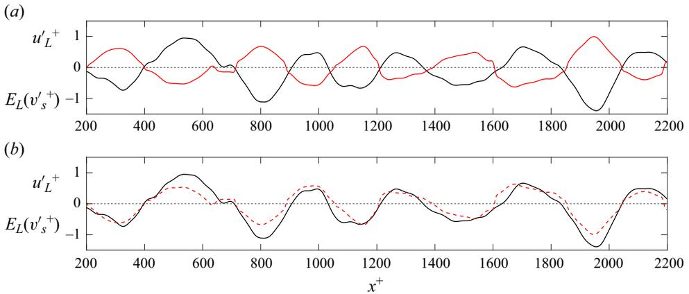
Figure 24. Amplitude modulation of  $v$  by  $u$ . Panel (a) shows large-scale streamwise velocity fluctuations (—) at  $y^+ \approx +5$  and the long-wavelength envelope of small-scale wall-normal velocity fluctuations (—, red) at  $y^+ = 0$  of case HP2; panel (b) shows the same, only with the envelope (—, red) now phase-shifted by  $\pi$ .
