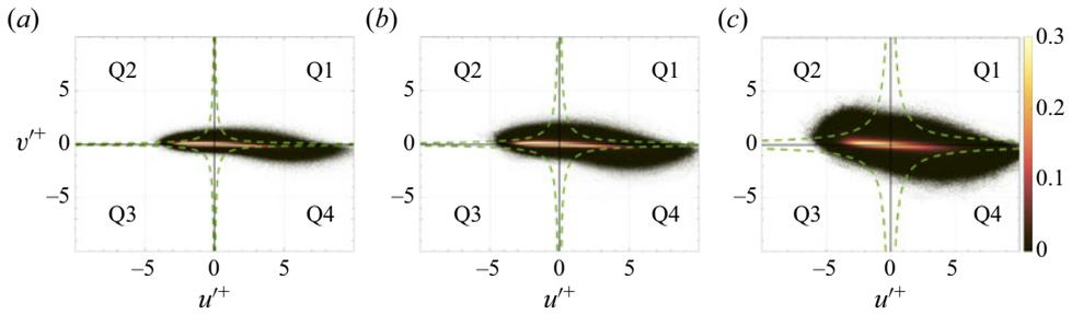
Figure 10. Quadrant maps of  $u'$  and  $v'$  at  $y^+ \approx 5$ : (a) smooth-wall, (b) LP1, (c) HP1. The dashed lines are hyperbolas marking  $|u'^+v'^+| = 8 \times -u'^+v'^+$ . The colour bar indicates the frequency of events in each bin of the map.
