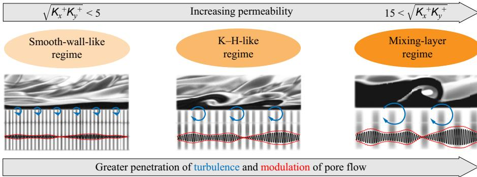
Figure 28. Conceptual sketch showing the evolution of turbulence over porous substrates. The lower limit  $\sqrt{K_x^+ K_y^+} < 5$  is based on (3.8) and the threshold shown in figure 9(d). The upper limit  $15 < \sqrt{K_x^+ K_y^+}$  is inferred from the results of Manes *et al.* (2011) in conjunction with (3.8).
