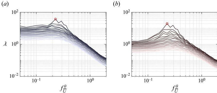
Figure 30. The SPOD eigenvalues of the (a) streamwise and (b) wall-normal velocity fluctuations at the surface ( $y^+ = 0$ ) of HP1. The peak in the leading SPOD mode at  $f = 0.22\bar{U}/\theta$  is circled in red. The shading of the curves varies from dark to light as the mode number increases.
