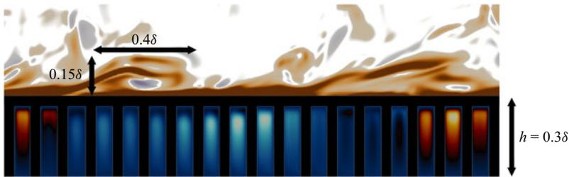
Figure 13. Vortex visualization using the  $Q$ -criterion above substrate HP1 in an  $x$ - $y$  slice through the simulation domain. Vortex cores (light colour) are regions of  $Q > 0$  (high vorticity) and surrounded by a sheet (dark colour) of  $Q < 0$  (high shear). The hot and cold regions below the surface represent positive and negative wall-normal velocity fluctuations, respectively. Flow direction is from left to right.
