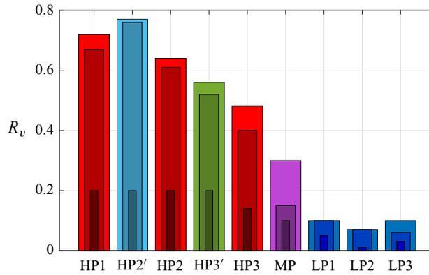
Figure 27. Degree of AM of the wall-normal velocity. Light to darker shades correspond to  $y^+ \approx -50$ ,  $y^+ \approx -110$  and  $y^+ \approx -110$ , respectively.
