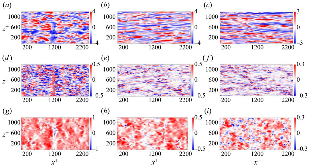
Figure 4. Instantaneous (*a–c*) streamwise velocity, (*d–f*) wall-normal velocity and (*g–i*) pressure fluctuations at  $y^+ \approx 5$ : (*a,d,g*) HP1; (*b,e,h*) LP1; (*c,f,i*) smooth-wall. Flow direction is from left to right.
