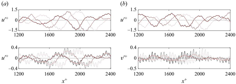
Figure 23. Raw (—) and low-pass filtered (—, red) spanwise-averaged velocity signals of case HP1: (a) streamwise velocity fluctuations at both  $y^+ \approx 5$  and  $y^+ = 0$ , (b) streamwise velocity fluctuations at  $y^+ \approx 5$  and wall-normal velocity fluctuations at  $y^+ = 0$ . The solid to faded lines represent three successive time signals.
