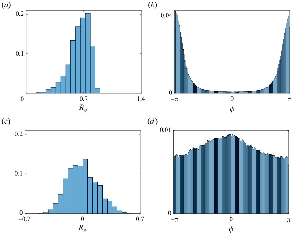
Figure 26. Probability density histograms of AM correlation between (a)  $u'_L{}^+$  and  $E_L(v'_s{}^+)$ , and (c)  $u'_L{}^+$  and  $E_L(w'_s{}^+)$ . Instantaneous phase differences between (b)  $u'_L{}^+$  and  $v'_L{}^+$ , (d)  $u'_L{}^+$  and  $w'_L{}^+$  for case HP2. The  $u'$  signal was taken at  $y^+ \approx 5$  while the  $v'$  and  $w'$  were taken at  $y^+ = 0$ .
