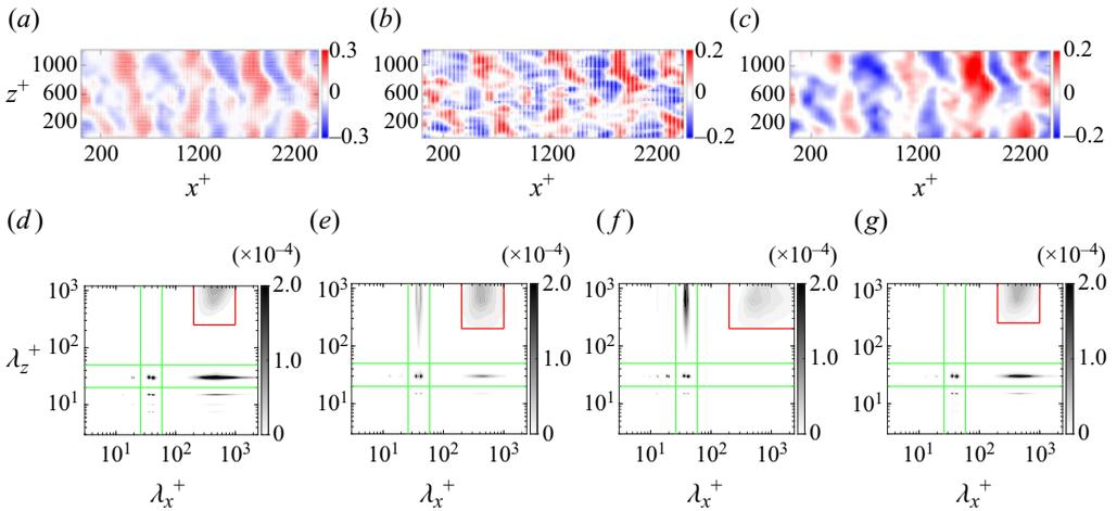
Figure 21. Instantaneous velocity fluctuations and premultiplied spectral energy densities of case HP1 at  $y^+ \approx -55$ : (a) streamwise fluctuations, (b) wall-normal fluctuations, (c) pressure fluctuations; (d)  $k_x k_z E_{uu}$ , (e)  $k_x k_z E_{vv}$ , (f)  $k_x k_z E_{ww}$  and (g)  $k_x k_z E_{uv}$ . The green lines enclose the most energetically significant parts of the pore-coherent flow and the red lines the surviving turbulence belonging to the K–H-like scales.
