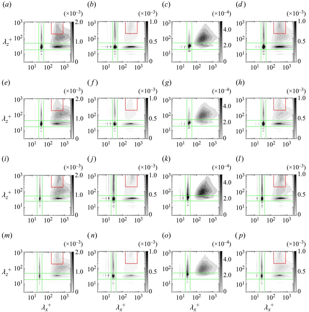
Figure 33. Premultiplied two-dimensional spectral densities: (a,e,i,m)  $k_x k_z E_{uu}$ ; (b,f,j,n)  $k_x k_z E_{vv}$ ; (c,g,k,o)  $k_x k_z E_{ww}$ ; (d,h,l,p)  $k_x k_z E_{uv}$  at  $y^+ = 0$ . Here (a–d) case HP2; (e–h) case HP3; (i–l) case HP2'; (m–p) case HP3'. The green lines enclose the most energetically significant parts of the pore-coherent flow and the red lines those of the K–H-like rollers.
