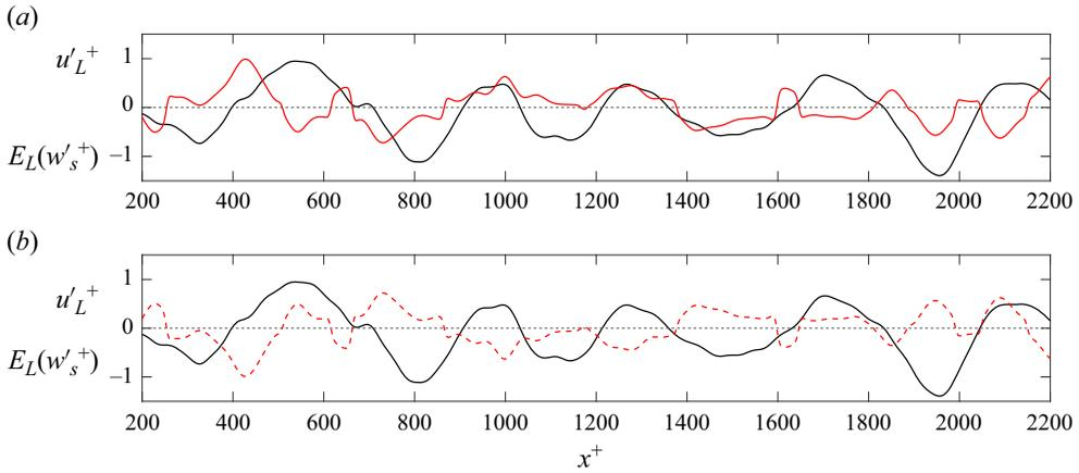
Figure 25. Lack of AM of  $w$  by  $u$ . The plots are similar to those in figure 24, but with the envelope of the spanwise velocity instead of the wall-normal velocity.
