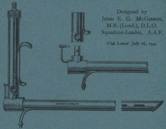
A Bronchoscope self contained with battery in handle, dispensing with entangling cables.
