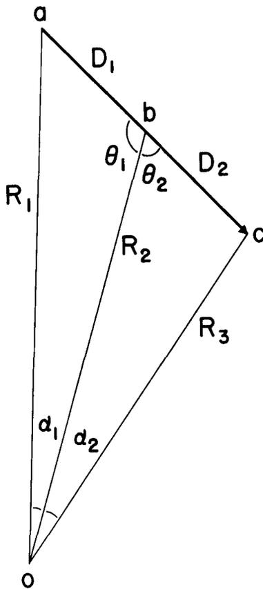
FIGURE 2.—Plane triangles formed by the meteor's trajectory and the observing station. The meteor was at  $a, b$ , and  $c$  at epochs 1, 2, and 3 respectively and at ranges  $R_1, R_2$ , and  $R_3$ , respectively. The observed angular lengths of the corresponding segments of the trail are  $\alpha_1$  and  $\alpha_2$ .
