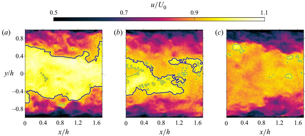
Figure 6. Sample instantaneous streamwise velocity fields for case C, showing (a) a continuous core, (b) a discontinuous core and (c) a ‘No QC’ example. Contour lines of  $u_{th} = 0.95U_0$  are indicated with blue lines. The thicker lines highlight the QC boundary.
