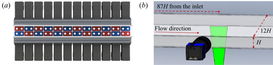
Figure 1. Schematic of (a) the active grid, and (b) the measurement set-up.
