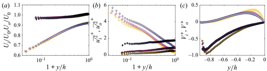
Figure 13. Weighted average profiles by  $\gamma$ , i.e. inside the core (symbols with black border), and by  $(1 - \gamma)$ , i.e. outside of the core (open symbols) of (a) mean streamwise velocity, (b) streamwise turbulent fluctuations and (c) mean vertical velocity for cases REF ( $\blacktriangleright$ , yellow), A ( $\blacksquare$ , orange), B ( $\bullet$ , purple) and C ( $\blacklozenge$ , navy blue).
