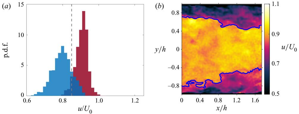
Figure 8. (a) p.d.f.s of the first (crimson), and the second (blue) modal velocity found for ‘No QC’ fields of case C with varying the streamwise domain from  $0.2h$  to  $1.7h$ . The grey dashed line marks  $u = 0.85U_0$ . (b) The same field as illustrated in figure 6(c) with contour lines of  $u_{th} = 0.85U_0$  delineating the new (low-momentum) core boundaries.
