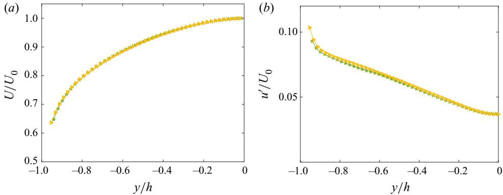
Figure 2. (a) Mean velocity, and (b) streamwise turbulence intensity profiles normalized by the centreline mean velocity for REF at  $X/H = 87$  ( $\blacktriangleright$ , yellow), and  $X/H = 100$  ( $\star$ , green).
