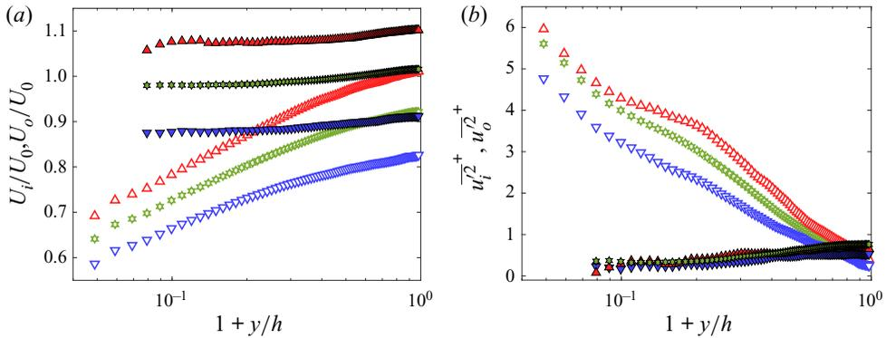
Figure 17. Weighted average profiles by  $\gamma$ , i.e. inside the core (symbols with black border), and by  $(1 - \gamma)$ , i.e. out of the core (open symbols) of (a) mean streamwise velocity, and (b) streamwise turbulent fluctuations for LMCs ( $\blacktriangledown$ , blue), OCs ( $\star$ , green) and HMCs ( $\blacktriangle$ , red) of case C.
