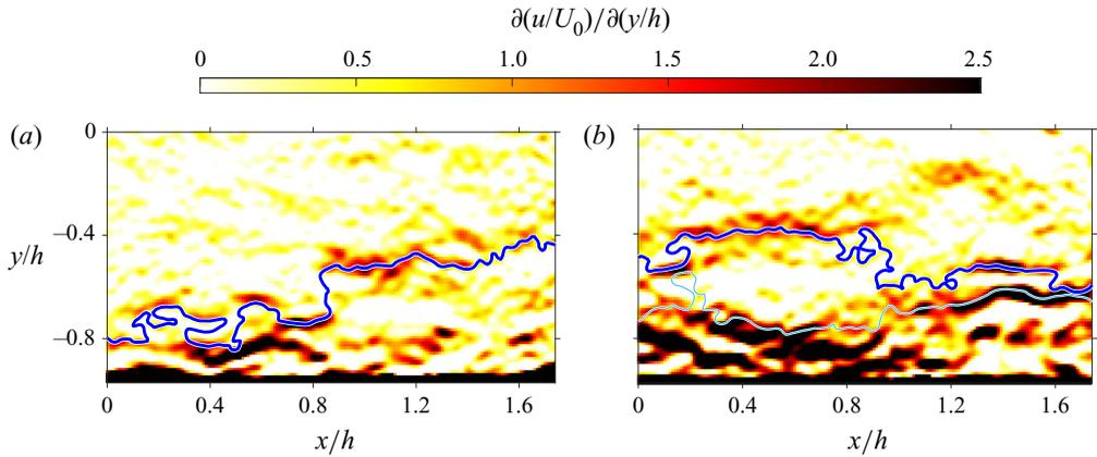
Figure 10. Instantaneous fields of streamwise velocity gradient in the lower half of the channel for the same field as (a) figure 8(b), and (b) figure 9(b). The thick blue line identifies the new core boundary. The thin blue line indicates the previously identified core boundary using  $u_{th} = 0.95U_0$ .
