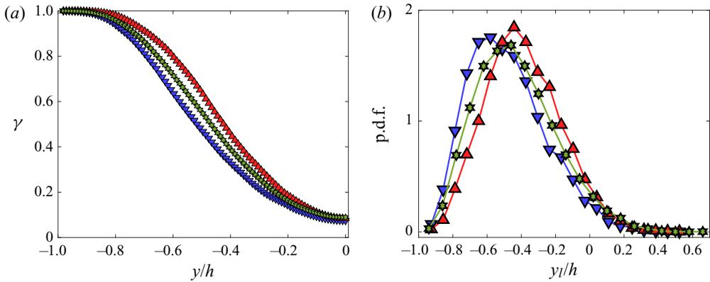
Figure 16. (a) Intermittency ( $\gamma$ ) profiles, and (b) p.d.f. of the core's lower boundary location for LMCs ( $\nabla$ , blue), OCs ( $\star$ , green) and HMCs ( $\blacktriangle$ , red) of case C.
