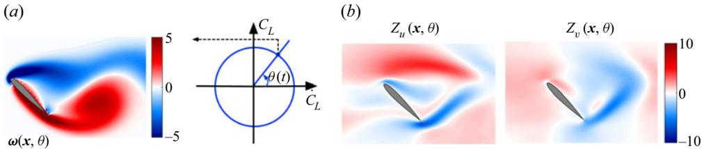
Figure 2. An overview of the phase reduction approach for flow over a NACA0012 airfoil at  $\alpha = 45^\circ$  and  $Re = 100$ . (a) Definition of phase based on the lift coefficient,  $C_L - \dot{C}_L$  plane. (b) Instantaneous spatial phase sensitivity fields  $Z_u$  and  $Z_v$  with respect to the perturbations in velocity fields.
