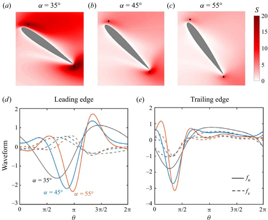
Figure 3. (a–c) Synchronization speed  $S$  around a NACA0012 airfoil at  $\alpha = 35^\circ$ ,  $45^\circ$  and  $55^\circ$ . The black dots indicate local maxima. (d–e) Theoretical optimal waveforms for fast synchronization with pointwise forcing at the leading and trailing edges for  $\alpha = 35^\circ$ ,  $45^\circ$  and  $55^\circ$ .
