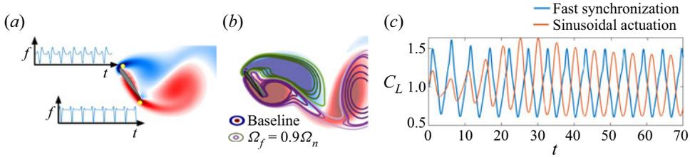
Figure 1. Fast synchronization analysis of flow over a NACA0012 airfoil at  $\alpha = 55^\circ$  and  $Re = 100$ . (a) Periodic actuation using the optimal waveform. (b) Comparison of the synchronized flow field for a forcing frequency  $\Omega_f = 0.9\Omega_n$  with the baseline vorticity field  $\omega$ . (c) Lift coefficient  $C_L(t)$  when actuated with the fast synchronization and sinusoidal waveforms.
