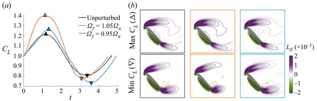
Figure 5. Characterization of  $C_L$  for the NACA0012 airfoil at  $\alpha = 45^\circ$  and  $Re = 100$ . (a) Variation of  $C_L$  when actuated with forcing frequencies  $\Omega_f = 1.05\Omega_n$  and  $0.95\Omega_n$ . (b) Instantaneous lift force elements  $L_E$  are shown for the actuated and unperturbed cases at max  $C_L$  ( $\Delta$ ) and min  $C_L$  ( $\nabla$ ).
