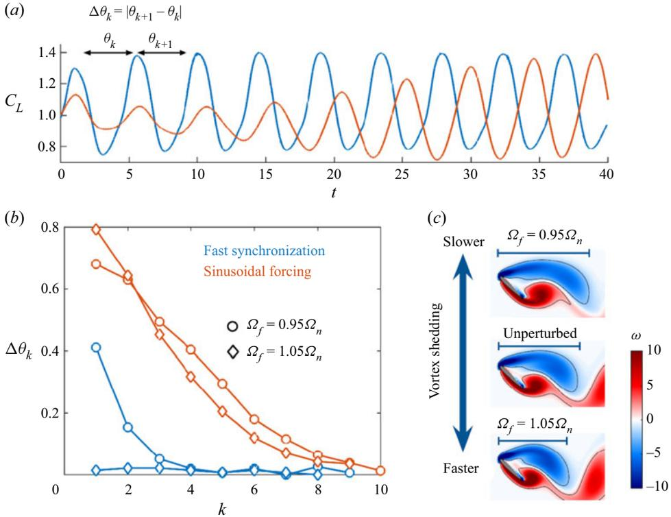
Figure 4. Numerical results for synchronization analysis of the NACA0012 airfoil at  $\alpha = 45^\circ$ . (a) Changes in  $C_L(t)$  at a forcing frequency  $\Omega_f = 1.05\Omega_n$ . (b) Synchronization time using sinusoidal and optimal waveforms at different forcing frequencies. (c) Comparison of instantaneous vorticity fields for forcing frequencies,  $\Omega_f = 0.95\Omega_n$  and  $\Omega_f = 1.05\Omega_n$  with the unperturbed vorticity field.
