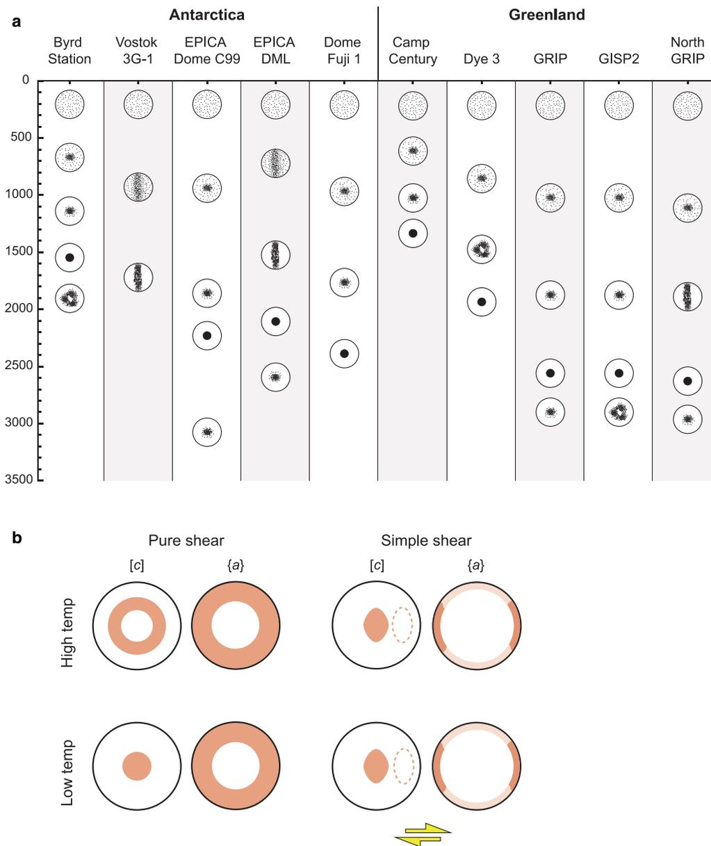
**Fig. 1.** Common CPO patterns in ice. (a) Empirical CPO observations from ice cores (001 axis only). Modified from Faria and others (2014). (b) Synthesis of common CPO patterns from both natural and experimental studies (refer text for references).
