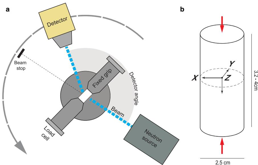
**Fig. 2.** (a) Experimental set-up for combined axial compression deformation and in situ CPO acquisition using neutron diffraction. (b) Orientation of  $D_2O$  samples during deformation experiments. Red arrows signify the shortening axis.
