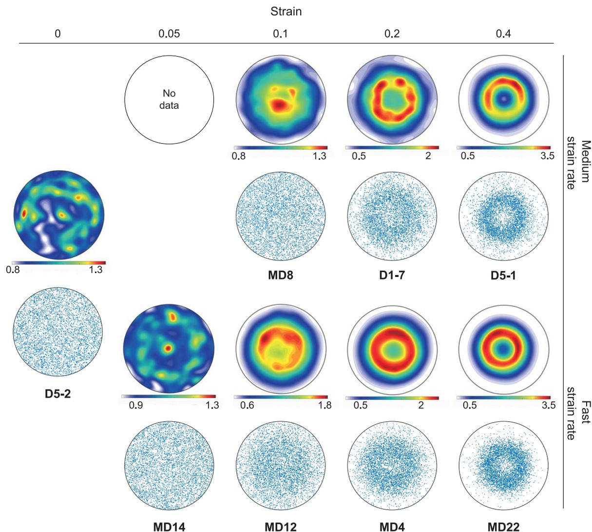
**Fig. 3.** Characteristic *c*-axis CPO patterns for various strains and strain rates. The shortening axis is parallel to the pole figure centre. At zero and low strains, a random distribution characterises the sample. With increased strain, the pattern changes from a weak cluster to a well-defined small circle parallel with the shortening axis, or 'cone'. Point plots were constructed using random orientations ( $n = 10\,000$ ) from the ODF.
