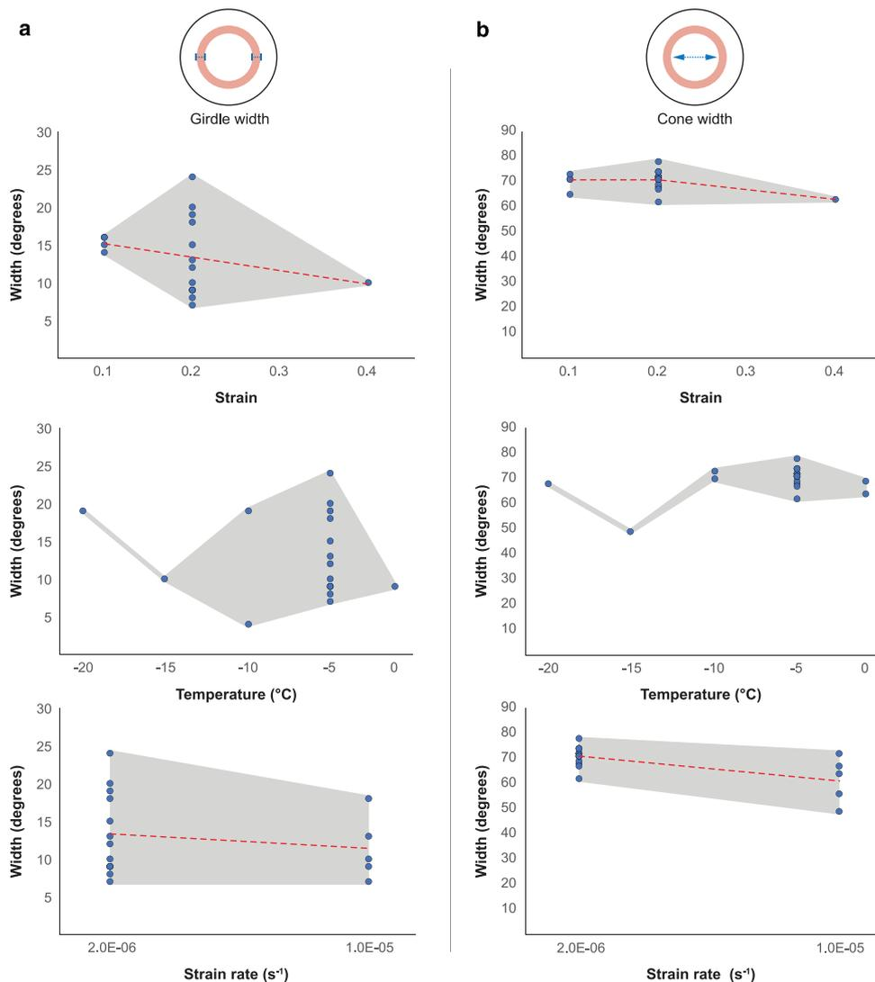
**Fig. 7.** Influence of increased strain, strain rate and temperature on (a) girdle width and (b) cone width. Strain data are from experiments at  $-7^{\circ}\text{C}$ . Temperature data are from experiments at 20% strain. Refer insets for visual definitions of girdle and cone widths.
