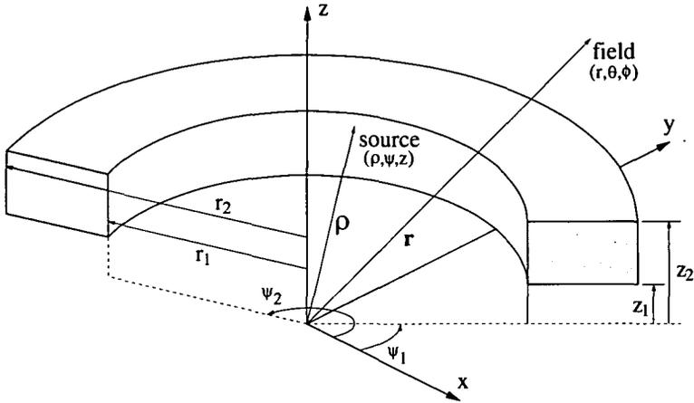
FIGURE 1. A typical circular arc with rectangular cross-section. Indicated are a source point  $\rho$ , measured in cylindrical polar coordinates, and field point  $r$ , measured in spherical polar coordinates.
