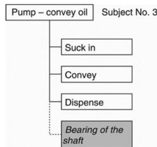
Fig. 4. Example function model for a hydraulic pump (Eckert et al., 2011).
