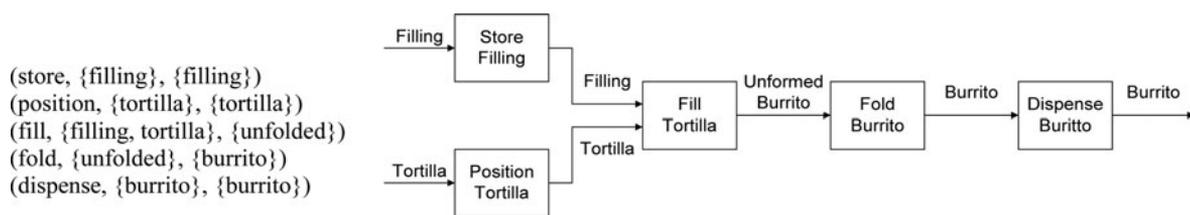
Fig. 5. Function list and function structure for burrito folder (Richardson et al., 2011).
