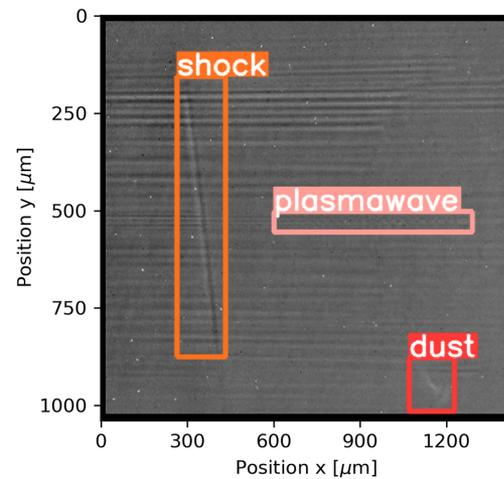
**Figure 10.** Machine learning application in few-cycle probing in a hybrid<sup>[21]</sup> laser-plasma accelerator. The objects to be detected in the shadowgram are the plasma wave, the shock and the diffraction patterns from dust particles.
