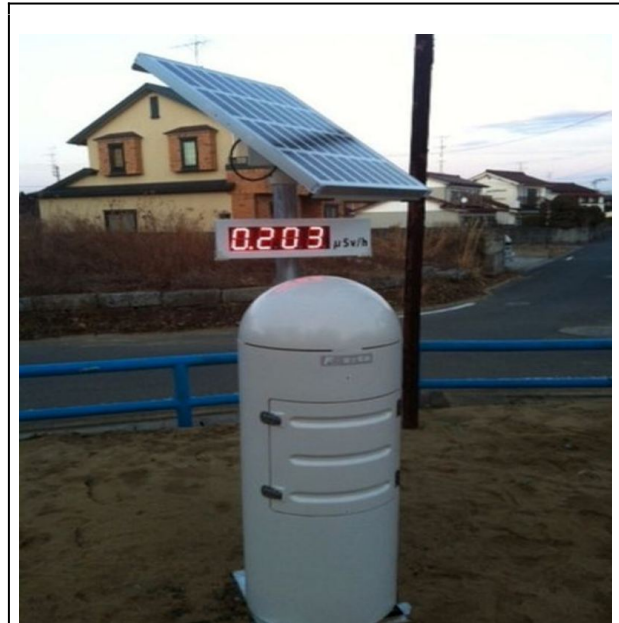
Radiation Monitoring Post (Minami-Soma, Fukushima) (Source)
