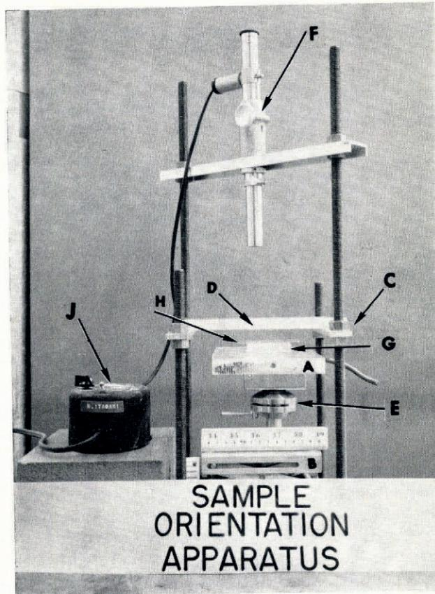
Fig. 1. Step one: ice sample orientation. *A*—moveable platform. *B*—laboratory jack. *C*—fixed supports. *D*—"Lucite" plate. *E*—rotatable head. *F*—telescope. *G*—ice sample. *H*—microscope slide. *J*—transformer.
