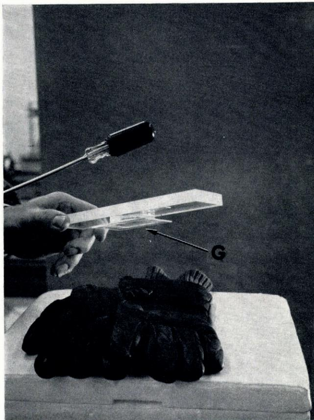
*Fig. 4. Step four: tapping the ice sample G free from the "Lucite" plate.*
