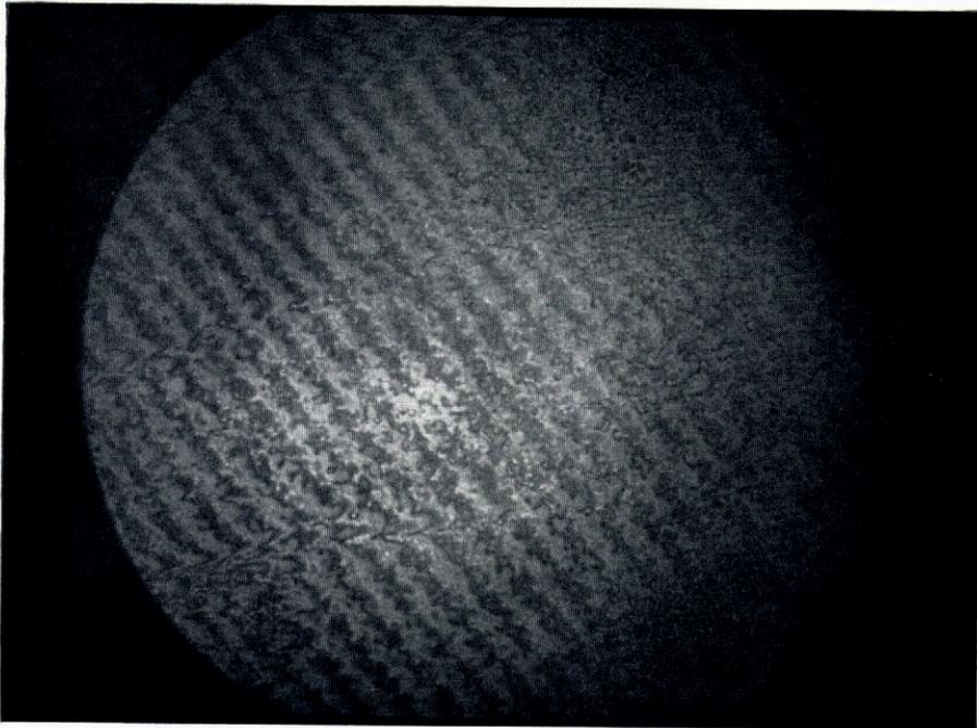
*Fig. 6. Interferogram of ice surface two hours after tapping.*
