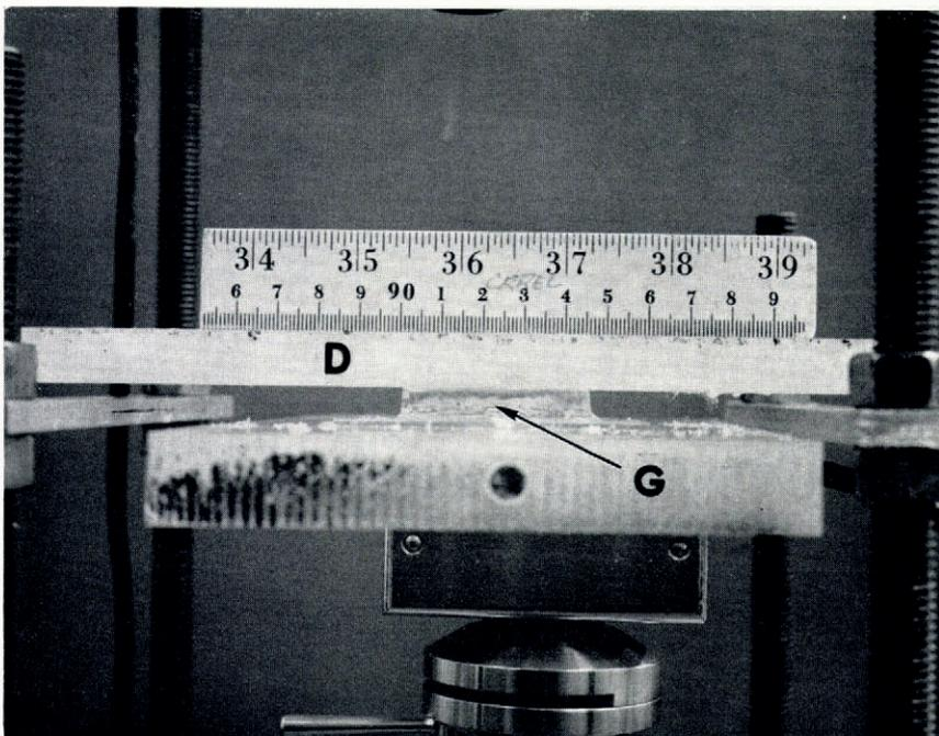
*Fig. 3. Step three: freezing the ice sample G to the "Lucite" plate D.*
