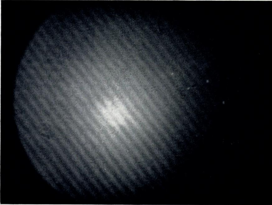
*Fig. 5. Interferogram of ice surface immediately after tapping.*
