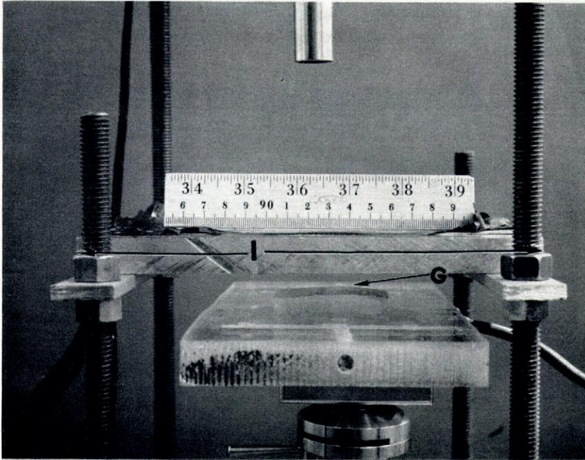
*Fig. 2. Step two: melting top layer of the ice sample G with aluminum heat slab I.*
