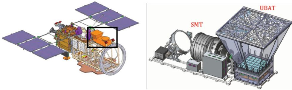
**Figure 6.** The integrated UFFO-pathfinder, to be launched aboard the *Lomonosov* spacecraft. The SMT enclosure is not shown in this drawing. Adapted from Chen *et al.* (2011).
