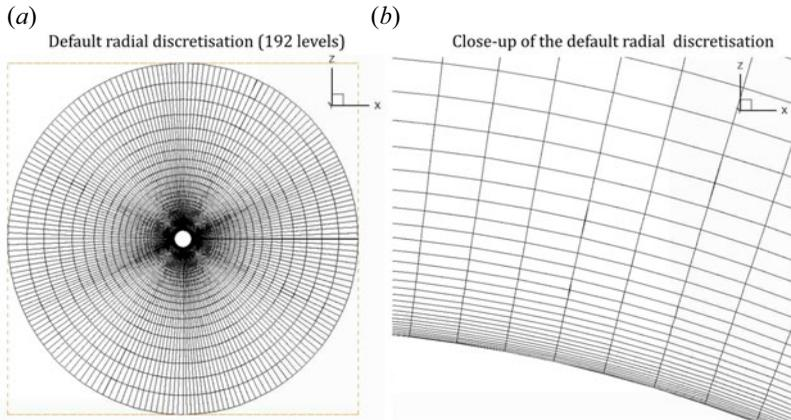
FIGURE 6. Illustration of the radial discretisation for the grids #1 and #2 and an enlarged view near the inner boundary.
