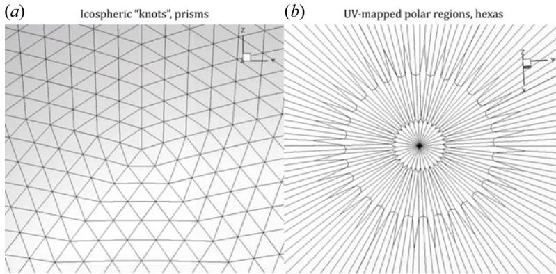
FIGURE 7. Non-uniformity regions in the two grid topologies. (a) The *knot* region in the icospheric grid is shown. This is the place where, in a Goldberg polyhedron, a pentagon would be located instead of a hexagon (and equivalently, here, the node only neighbours five other nodes instead of six). (b) The distorted polar regions of the *UV*-mapped mesh are shown, where originally the degenerated prisms were placed.
