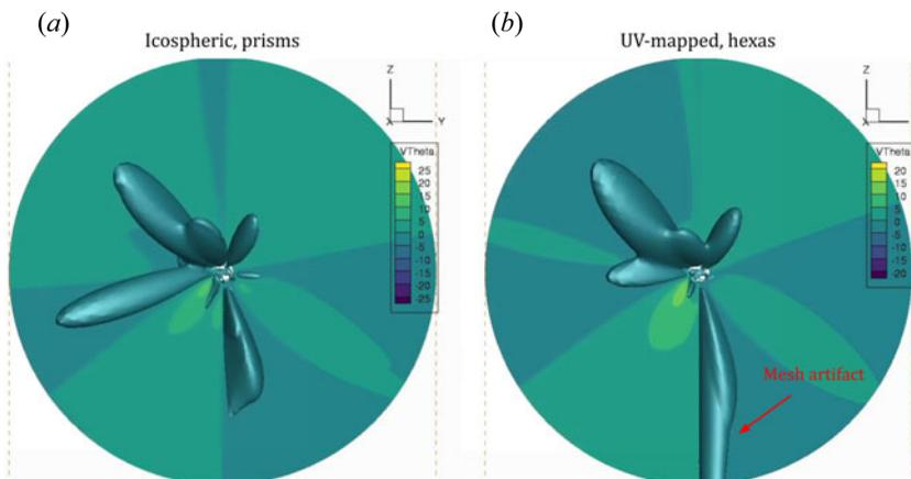
FIGURE 16. The  $-2.5 \text{ km s}^{-1}$  isosurface in  $V_\theta$ , showing that in this case, when the flow features are also present near the polar regions, the  $UV$  mesh with high distortion in these zones also creates very strong artefacts (b).
