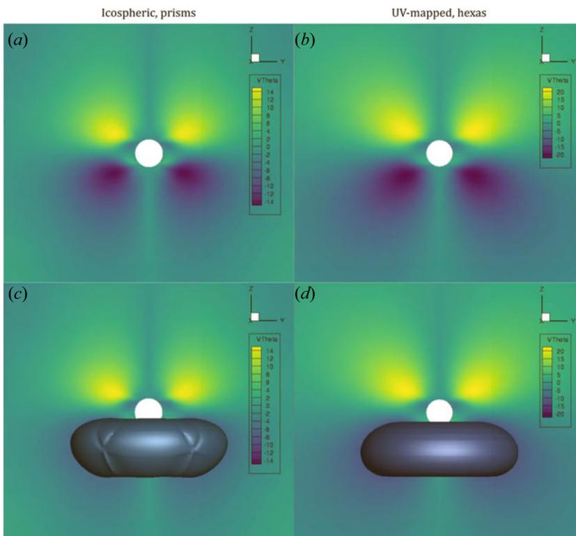
FIGURE 10. Comparison of the  $V_\theta$  solution fields of a rotating dipole for (a), (c) the icosaheric, prism-based mesh and (b), (d) the  $UV$  mesh with hexahedrons. Although the solution projected onto the  $X$  axis looks similar, the isosurfaces of  $V_\theta$  ( $-9 \text{ km s}^{-1}$ ) show that the icosaheric mesh produces mesh artefacts around the regions where the knots are present in the grid and where they are connected together.
