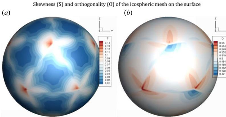
FIGURE 8. Skewness and orthogonality of the icospheric mesh, showing how these two quantities change around the mesh knots.
