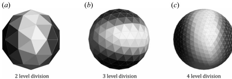
FIGURE 3. Principle of surface element splitting to achieve a finer and better-approximated spherical surface for the geodesic polyhedron. Each next level has four times as many elements on the surface as the previous level. The division level for the grids used in this paper for the dipole and magnetogram simulations was six.
