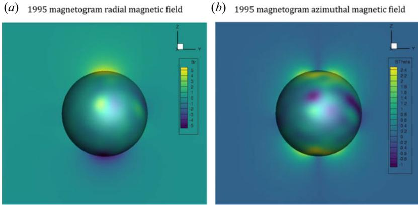
FIGURE 17. Radial and azimuthal components of the magnetic field,  $B_r$  and  $B_\theta$ , applied on the inner boundary based on the solar magnetogram from 1995.
