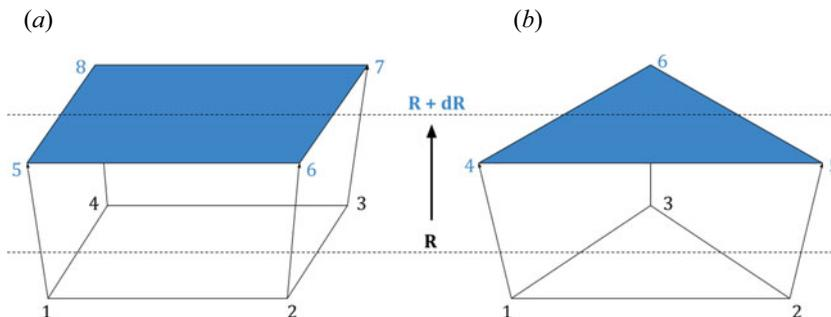
FIGURE 5. Principle of the extension of the spherical grids into a 3D domain applied in this work. The radial discretisation (from  $R$  to  $R + dR$ ) is independent of the selected topology. The 3D element is constructed using the original surface element (white), the extended surface element (blue) and the walls created by the radial extrusion.
