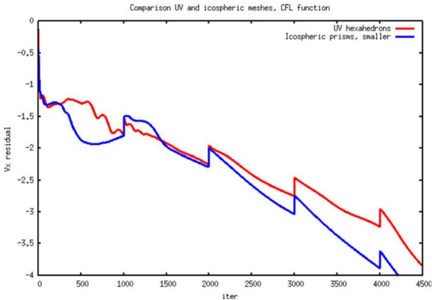
FIGURE 21. Comparison of the convergence history for the 1999 magnetogram in  $V_x$  ( $x$  component of the velocity) for the  $UV$  mesh (#1) and the coarser icospheric mesh (#3). The ripples in the convergence curves are caused by the doubling of the CFL every 1000 iterations. Here, the icospheric mesh reaches the target residual earlier than mesh #2 from figure 20 thanks to a more comparable mesh-associated numerical dissipation.
