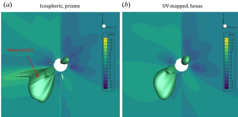
FIGURE 15. The  $1.5 \text{ km s}^{-1}$  isosurface of  $V_\phi$ , showing the mesh lines in the case of (a) the icospheric grid and (b) a relatively clean solution of the  $UV$  grid. The two results are not completely equivalent because owing to the different mesh topologies, the latitudinal and longitudinal resolution is significantly different.
