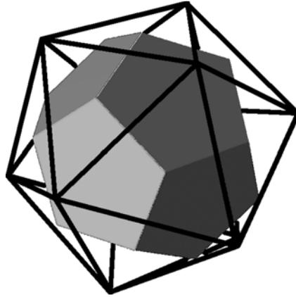
FIGURE 1. Comparison between the Goldberg polyhedron (solid) with hexagons and pentagons and the geodesic polyhedron (wireframe) with triangular elements. The Goldberg polyhedron is the dual of the geodesic polyhedron and vice versa.
