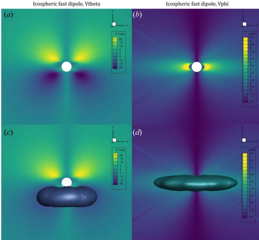
FIGURE 13. The  $V_\theta$  and  $V_\phi$  solution field  $X$ -plane projections and isosurfaces for a fast rotating dipole when the icospheric mesh is applied. It can be observed that when the dynamics in the solution is stronger (here the prescribed  $V_\phi$  had double the magnitude compared with figures 11 and 10), the mesh artefacts are weaker in the relative sense.
