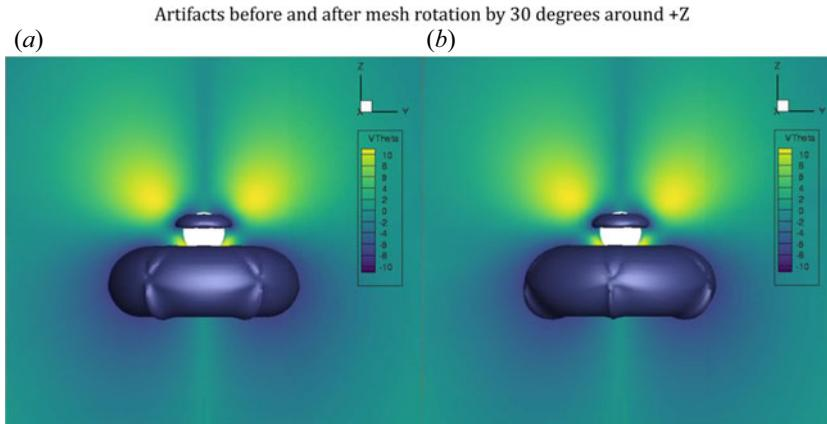
FIGURE 22. Comparison of the  $V_\theta$  artefacts in the solution of the dipole before and after the mesh is rotated by  $30^\circ$  around the  $Z$  axis. The artefacts are now located at different places, allowing the user to identify these features as indeed being mesh-related and analyse the local solution field without the effects of these artefacts.
