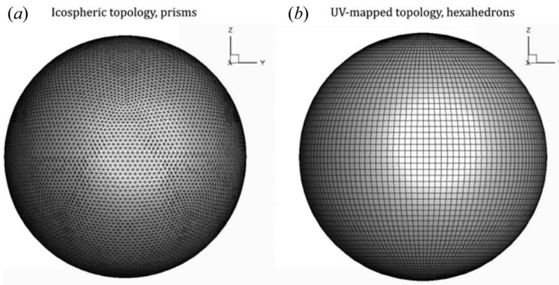
FIGURE 4. The two main surface topologies used to generate 3D meshes for the coronal MHD simulations: the level-six divided geodesic polyhedron (an *icosphere* from here on) and the *UV*-mapped sphere (a *UV sphere* from here on).
