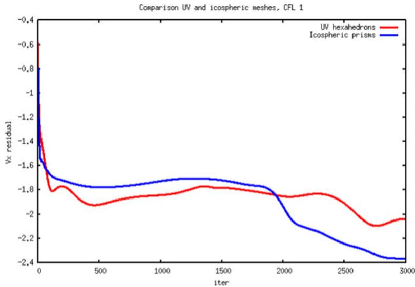
FIGURE 19. Comparison of a partial convergence history for the 1999 magnetogram in  $V_x$  ( $x$  component of the velocity) for the  $UV$  mesh (#1) and the fine icospheric mesh (#2) with a CFL of 1. The beginning of the convergence history is shown to display the effect of the polar regions resulting in the residual oscillations in case of the  $UV$  mesh from the iteration 2000 onward.
