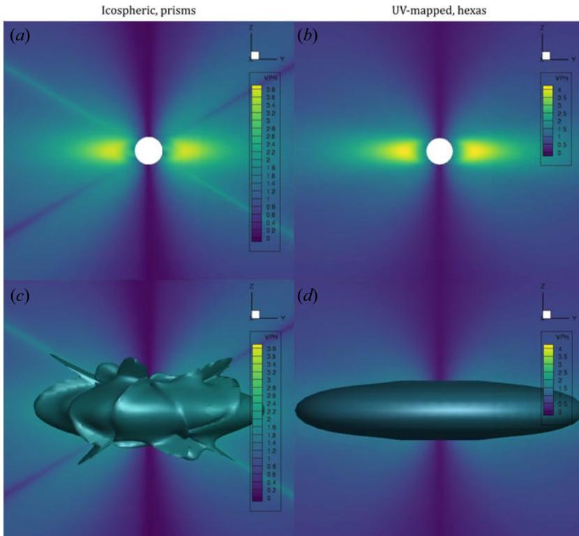
FIGURE 11. Comparison of the  $V_\phi$  solution fields of a rotating dipole for (a), (c) the icospheric, prism-based mesh and (b), (d) the UV mesh with hexahedrons. In this case, the mesh artefacts from the knots and knot lines in the icospheric mesh are already observable in the projected field and the isosurface of  $V_\phi$  (roughly  $-1.5 \text{ km s}^{-1}$ ) is highly distorted.
