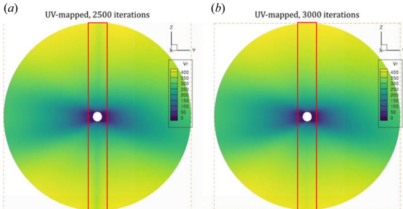
FIGURE 18. Display of the convergence challenges of a coronal MHD simulation of the 1995 magnetogram when a mesh with highly distorted polar regions is used, in this case introducing spurious outflow during convergence.
