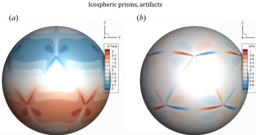
FIGURE 12. Projection of (a)  $V_\theta$  and (b)  $V_\phi$  icosahedric solutions onto the outer boundary to better illustrate the mesh artefacts. The artefacts are contained in the lines connecting the knots of the mesh.
