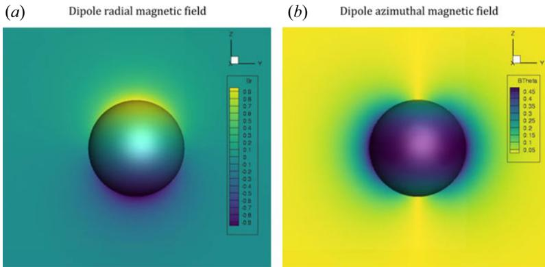
FIGURE 9. Configuration of the magnetic field to simulate the magnetic dipole, with (a) the radial component  $B_r$  and (b) the azimuthal component  $B_\theta$ .
