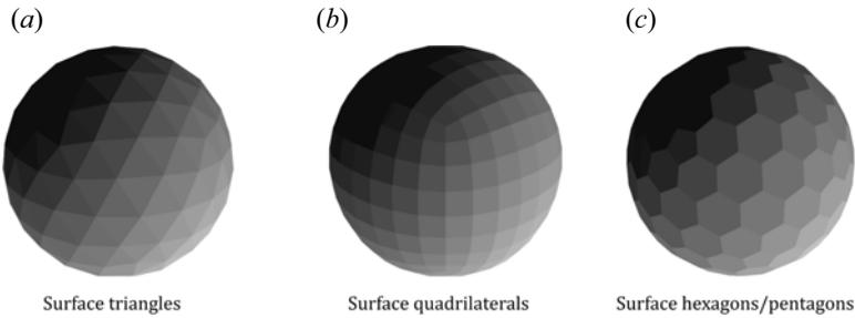
FIGURE 2. Three different configurations derived from the icosahedron-based spherical surface construction. In addition to the geodesic polyhedron and the Goldberg polyhedron, also an alternative with surface quadrilaterals is shown in (b). The latter configuration, however, resulted in much stronger mesh artefacts in the solution compared with the geodesic polyhedron due to higher skewness, so it is not investigated further in this paper.
