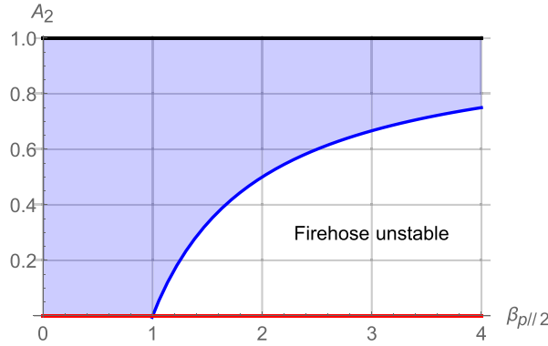
FIGURE 3. Stability diagram of Stage 1. Since T_{\perp 2} = 0 , it lies on the red line and is firehose stable within the shaded area.
