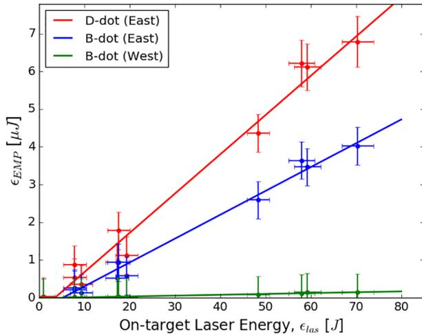
**Figure 2.** EMP energy versus on-target laser energy for the D-dot and two B-dot probes. The coloured lines represent linear fits for all three probes.
