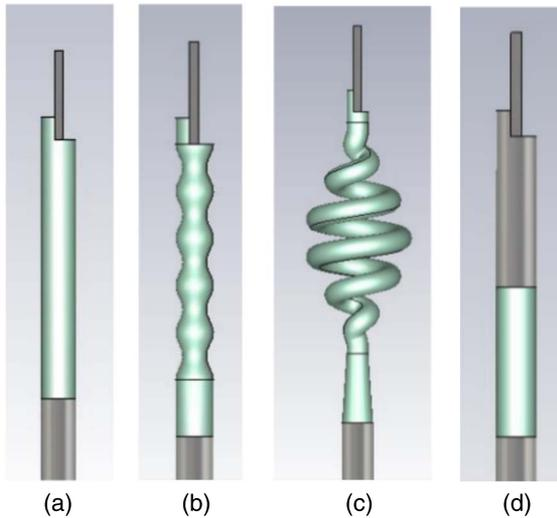
**Figure 11.** Side elevation of stalk designs used in 3D PIC simulations. Transparent grey sections represent a perfect electrical conductor (PEC), while the grey-green regions represent Teflon plastic. (a) Standard cylindrical stalk configuration: pure Teflon and PEC models were used. (b) Sinusoidally modulated Teflon stalk. (c) Teflon spiral stalk. (d) Half-length Teflon and PEC stalk.
