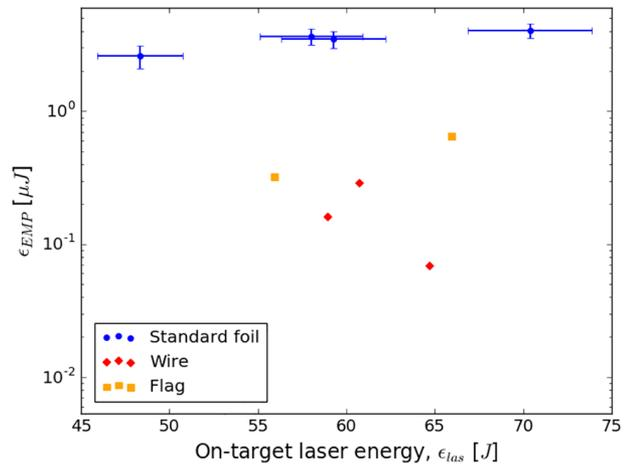
**Figure 6.** EMP energy as a function of on-target laser energy for wire, flag and standard foil designs (B-dot probe East). Laser focal intensity ranges from  $8 \times 10^{17} \text{ W} \cdot \text{cm}^{-2}$  to  $2 \times 10^{19} \text{ W} \cdot \text{cm}^{-2}$  on these shots and we have chosen a logarithmic y-axis to emphasize the drop in EMP. Notice how changing the wire diameter has led to a deviation from the linear relationship between EMP and on-target laser energy.
