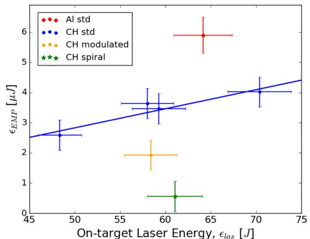
**Figure 7.** EMP energy versus on-target laser energy for a variety of different stalk designs (B-dot probe East). Laser focal intensity is between  $8 \times 10^{17} \text{ W} \cdot \text{cm}^{-2}$  and  $2 \times 10^{19} \text{ W} \cdot \text{cm}^{-2}$  for these shots. Also included is a linear fit to the standard CH cylindrical stalk data, as detailed in Figure 2.
