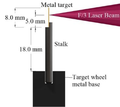
**Figure 1.** Schematic of target design and experimental arrangement.
