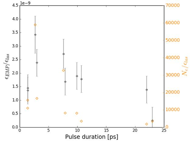
**Figure 3.** Plot of EMP energy and total number of escaping electrons versus laser pulse duration. The grey diamonds represent the ratio of EMP energy to on-target laser energy, while the orange diamonds represent the ratio of total electron number ( $N_e$ ) to on-target laser energy. EMP data was taken from the B-dot West probe.
