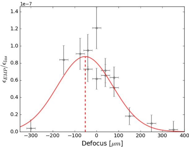
**Figure 5.** The ratio of EMP energy to laser energy plotted against defocus (as measured by the D-dot East probe). The Gaussian fit is meant as a visual aid, with a laser focal intensity of approximately  $1 \times 10^{18} \text{ W} \cdot \text{cm}^{-2}$  at the Gaussian peak.
