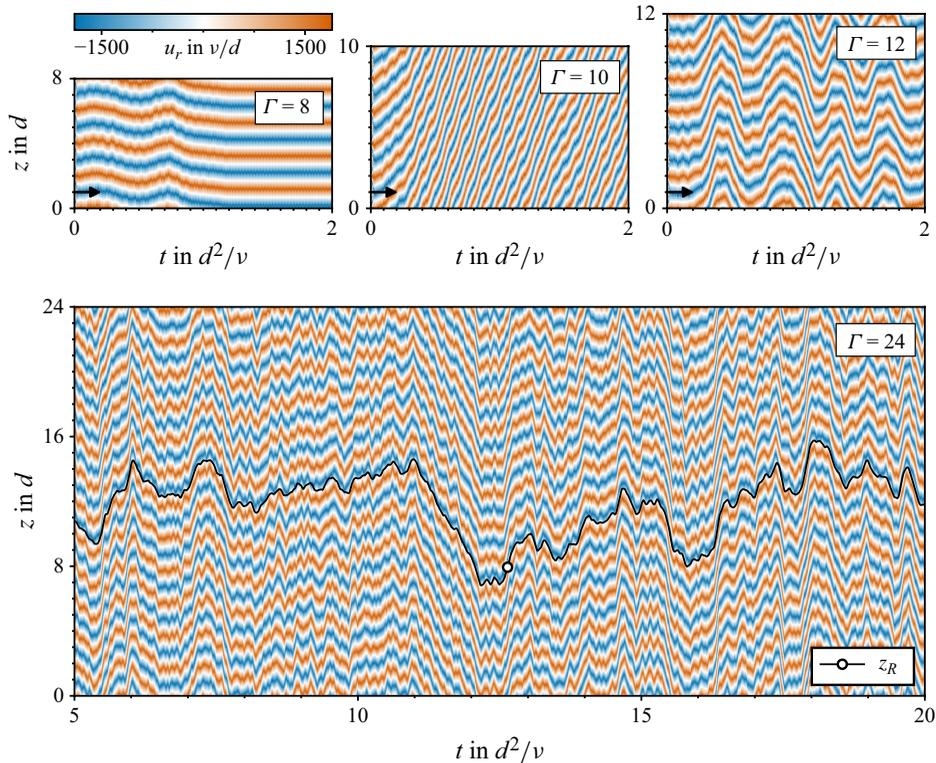
Figure 1. Temporal evolution of radial velocity along an axial line at mid-gap. The aspect ratio  $\Gamma$  of axial length to radial gap corresponds to the number of vortices. For  $\Gamma = 8$ , after an initial transient, the vortices do not move, while for  $\Gamma = 10$ , they move very quickly in one direction. For  $\Gamma = 12$  and 24, the vortices sporadically change their direction of motion. From Feldmann & Avila (2025).
