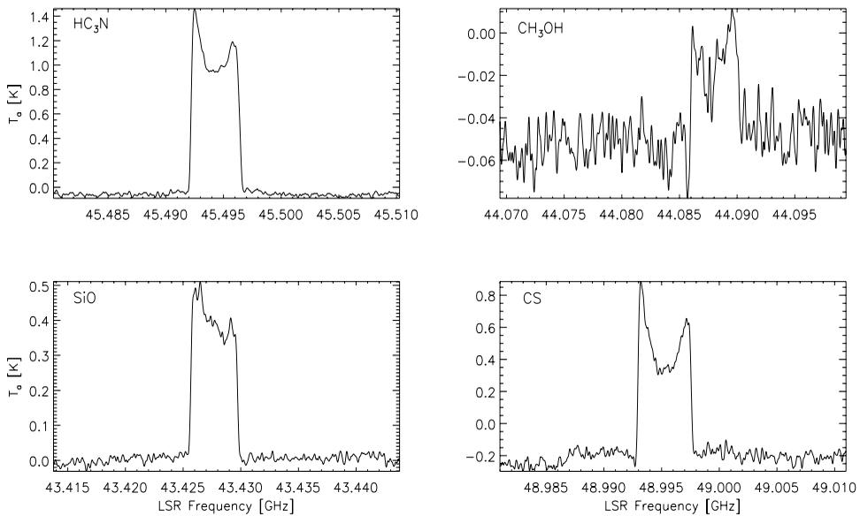
**Figure 1.** Spectra of several species in IRC+10216. The intensity scale has been calibrated in units of antenna temperature. We have not corrected for the atmosphere or removed the zero level in these “raw” spectra. The data have been smoothed to a velocity resolution of  $\sim 1 \text{ km s}^{-1}$ .
