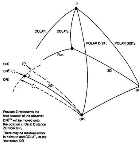
Fig. 1. Correction of zenith distance
