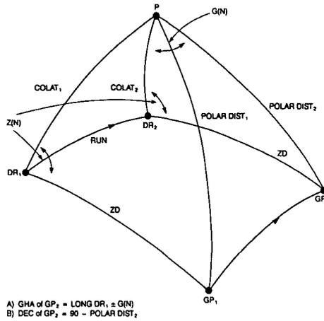
Fig. 2. Determination of transferred values of DEC and GHA
