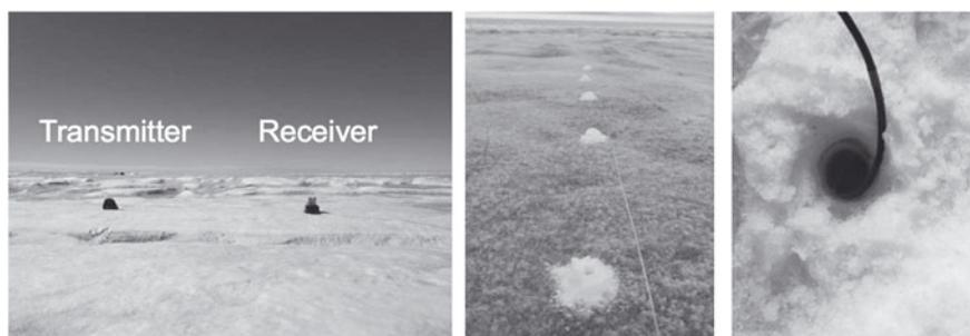
**Fig. 2.** An acoustic link through the Greenland ice sheet. The left-hand image shows the transmitter and receiver pair; the centre image shows a typical experimental configuration, in which a row of holes are drilled and the signal attenuation between these holes is measured; and the rightmost image shows an acoustic transducer in a flooded drilled hole.
