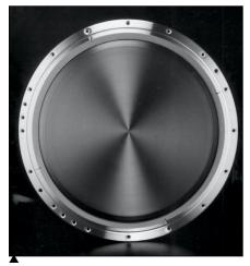
**Tantalum Targets:** Tosoh SMD offers tantalum targets that have a grain size of <65 μm with preferred grain orientation and a low oxygen content of <50 ppm. The material has a 4N5 purity with low nobium content and is available for all leading PVD systems. With high strength in excess of 20,000 psi, the tantalum target assembly uses Tosoh SMD's Prelude<sup>®</sup> diffusion bonding technology. Contact: portugaljv@tsmd.com; www.tsmd.com.
