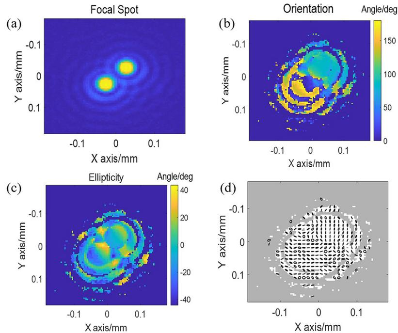
**Figure 6.** Focal spot after PS: (a) intensity distribution; (b) orientation of polarization calculated by Stokes parameters; (c) ellipticity; (d) polarization distribution.
