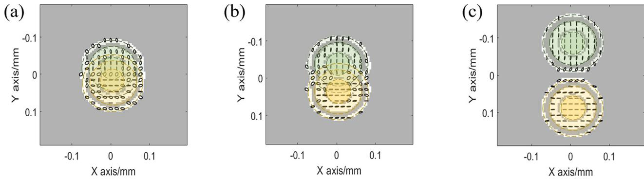
**Figure 3.** Polarization distribution within the focal point at various separation angles: (a)  $\alpha = \text{DL}$ ; (b)  $\alpha = 2\text{DL}$ ; (c)  $\alpha = 5\text{DL}$ .
