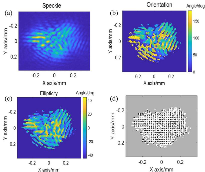
**Figure 7.** Speckle after the CPP and PS: (a) intensity distribution; (b) orientation; (c) ellipticity; (d) distribution of polarization states.
