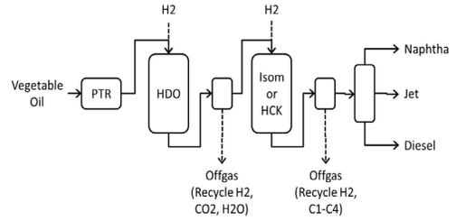
Figure 4. Schematic of representative HVO Plant.
