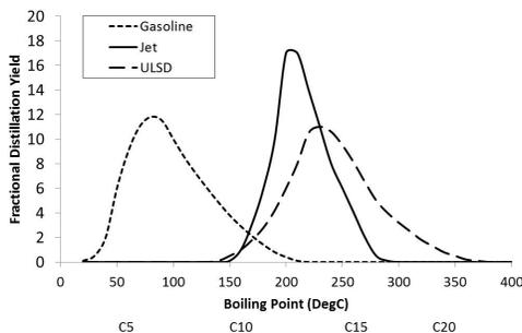
Figure 5. Representative boiling ranges of fossil gasoline, jet and diesel.
