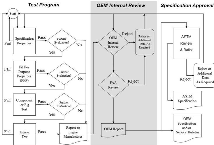
Figure 2. Overview fuel and additive approval process. (Reproduced by courtesy of ASTM)
