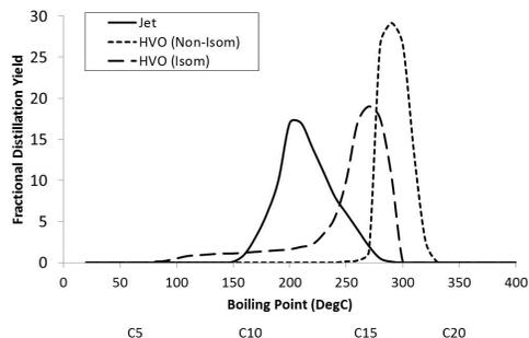
Figure 6. Representative boiling ranges of conventional jet, un-isomerised and isomerised hydrogenated vegetable oil.
