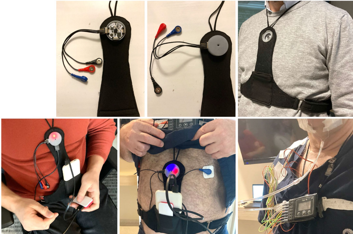
Figure 3. Performance tests and refinements, followed by controlled lab evaluations assessing respiratory and sleep-related variables
