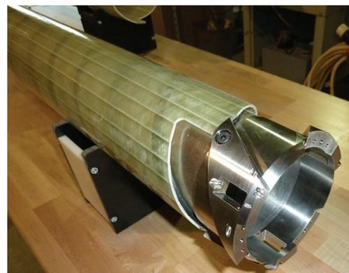
Fig. 8. Fiberglass outer tube with dry core barrel and cutter head.
