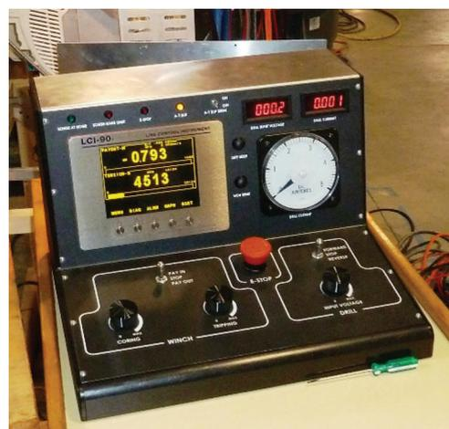
Fig. 10. Drill control console.
