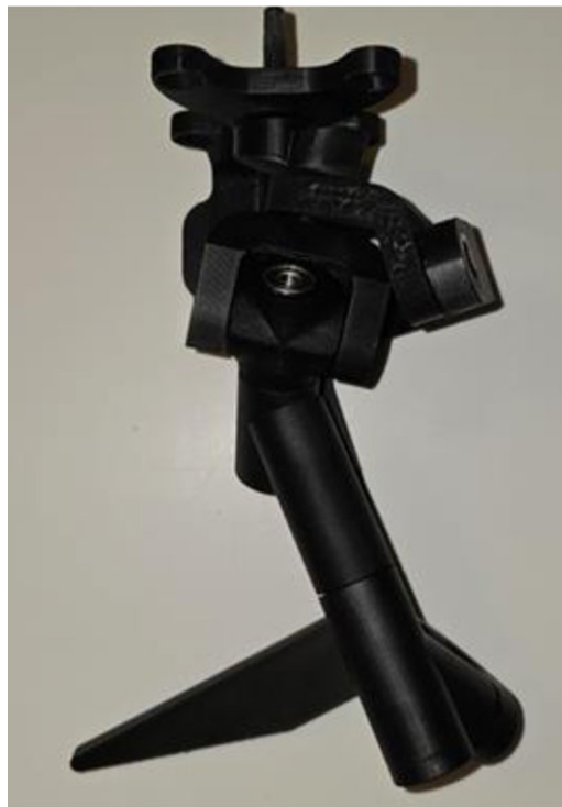
Figure 12. Assembled overconstrained walking mechanism.
