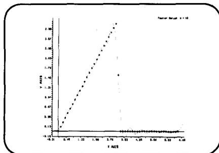
In a graphical display under the Fourier Series menu, the data points appear as circles and a fitted Fourier series of order ten is plotted as a dotted curve.
