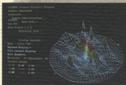
*Complete calculation of the full residual stress tensor using uniaxial, biaxial or triaxial stress calculations.*
