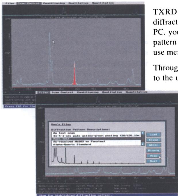
TXRD 3.5 brings you low cost semi-automation of manual diffractometers, but as a fully integrated analysis platform for the PC, you'll find it to be much more. All of your x-ray diffraction pattern analysis needs are a mouse click away with a simple-to-use menu-driven environment.
