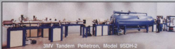
3MV Tandem Pelletron, Model 9SDH-2
