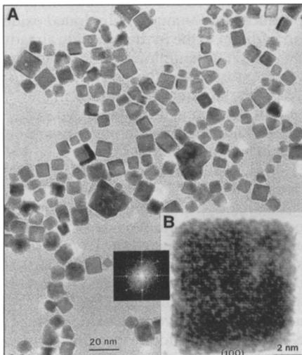
(A) Low-magnification transmission electron microscope (TEM) image of polymer-capped platinum nanoparticles from a solution with a 1:1 polymer to platinum cation ratio, showing the size and shape distribution of the cubic particles. (B) High-resolution lattice image of a cubic platinum particle. (Inset) The Fourier transform of the lattice image gives the optical diffractogram of the particle. (Photo courtesy of Science.)
