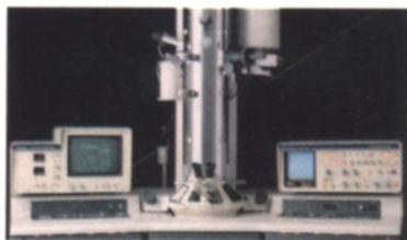
ity, accuracy and reliability. And the turbomolecular pump (TMP) and column-baking mode mean fast pumpdowns and clean vacuum conditions.
